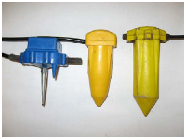
Figure 3.1. The three geophone cases used in the sensor test. Left: Oyo 3C, middle: ION Spike, right: Oyo Nail.
