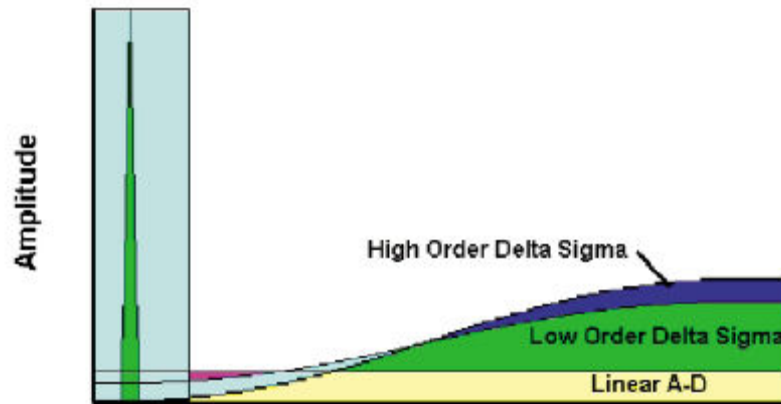
FIG 1.8. Noise shaping of Delta Sigma ADCs (Cooper, 2002). The shaded blue box on the left represents the desired frequency band, with the large green spike representing signal frequencies. Frequencies greater than the frequency band contain significantly more noise, but will be filtered prior to recording.
