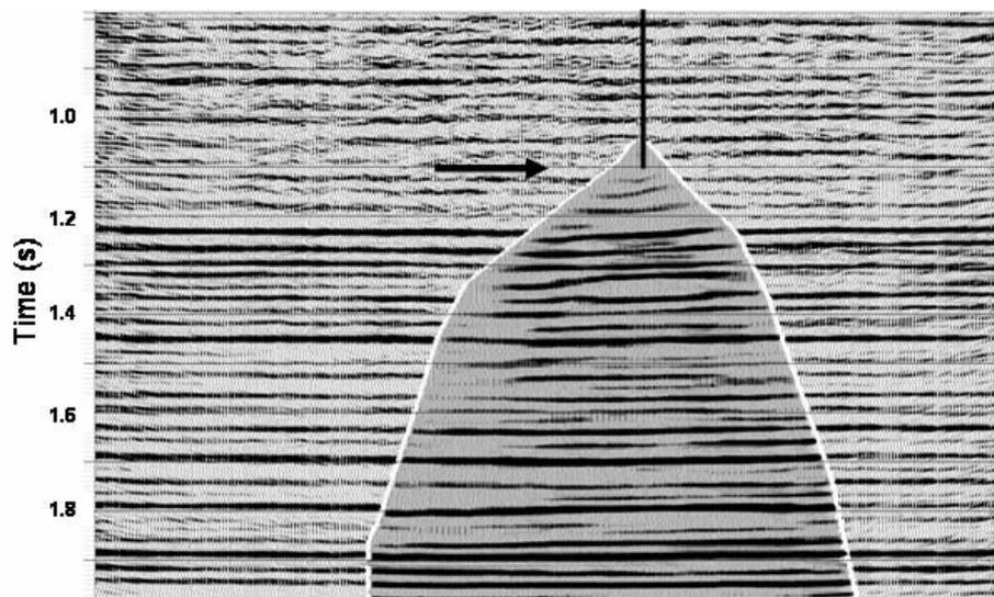
Figure 2. P-wave image across the injection pad. VSP data are spliced into the section. Cardium Formation is shown by the arrow; the observation well is indicated by the vertical line.
