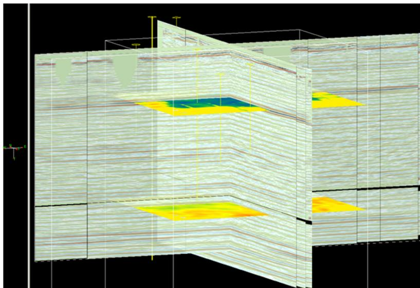
Figure 2. Slices from the P-wave volume imaged across the injection pad. The lower time slice correlates with the Cardium Formation.
