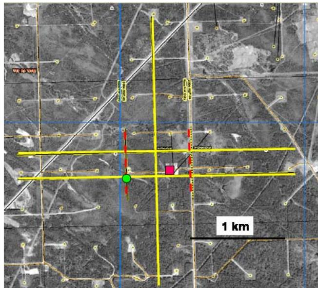
Figure 1. Map showing Penn West CO<sub>2</sub> injection site. Multicomponent seismic lines are shown in yellow, and receivers-only lines are shown in red. The observation (VSP) well is shown by the filled green circle, and the CO<sub>2</sub> injection pad is indicated by the red square.
