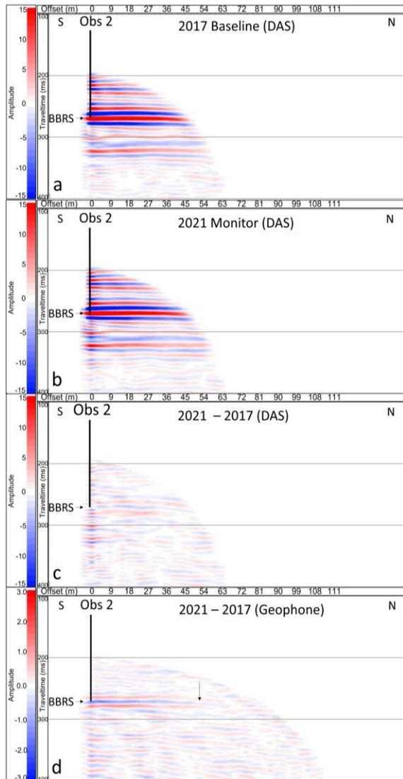
Figure 4: Baseline (a) and monitor (b) VSP CDP stacks of Line 7 DAS data. The time-lapse difference (c) does not clearly detect the CO<sub>2</sub> plume, as in the geophone result (d).
