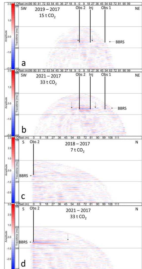
Figure 3: Time lapse results from Line 13 (a & b) and Line 7 (c & d) showing detection of the CO<sub>2</sub> plume after 33 t of injection.
