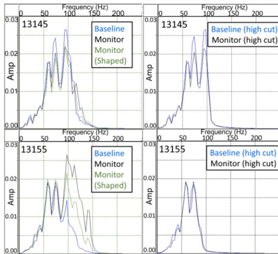
Figure 2: Baseline and monitor spectra from processed shot gathers. Shaping filters did not adequately address the variable near-surface filtering effects (left panels). After the application of high-cut filters (right panels), the baseline amplitudes could be directly subtracted from the monitor data.
