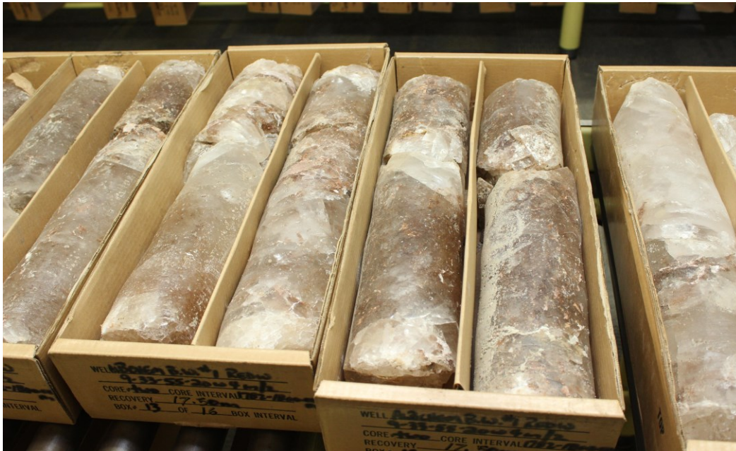
Figure 1. A core photo from the Lotsberg Formation Salt, TWP 55-20W4. This section was removed using solution mining to create the salt cavern.
