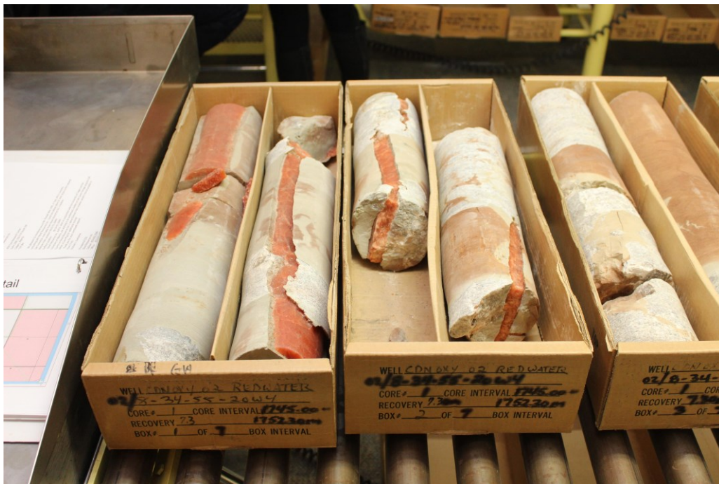
Figure 2. A core photo from the cap rock that seals the Lotsberg Formation Salt, TWP 55-20W4.
