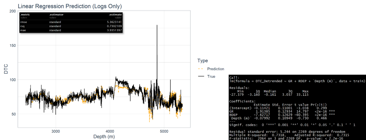
Figure 2: Baseline linear regression model using only RDEP, GR, and Depth to predict DTC.
