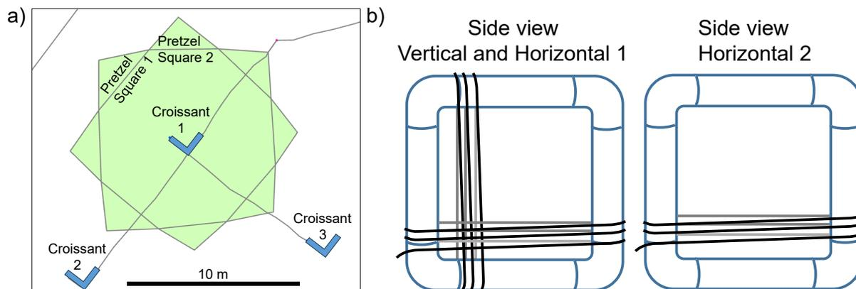
Figure 1. Map (a) showing Pretzel and Croissant locations (buried fiber locations are shown with grey lines), and a schematic (b) showing wrapped fiber orientation on two 1x1 m plastic frames that were installed vertically at each Croissant location (blue chevrons, Figure 1a).
