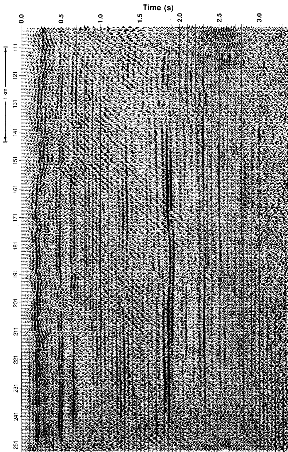
FIG. 6.12. Stack section of radial-component data with final vertical-component statics applied.
