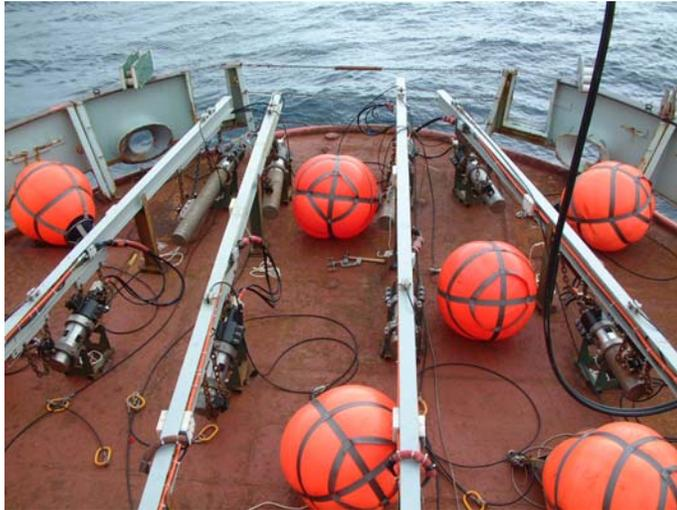
Figure 4.9: Air gun array. (Modified from Jackson et al., 2002)
