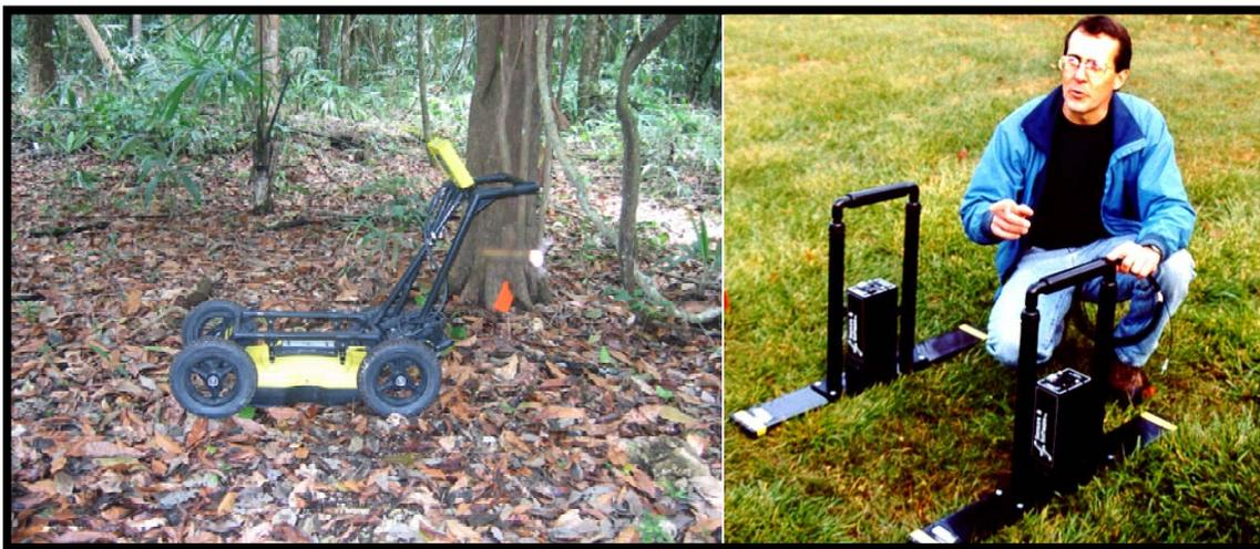
**Figure 3.1** Noggin 250 MHz Smart-cart unit (left); photo courtesy of R. Stewart, and the Pulse EKKO 100 MHz unit (right) ([www.eescience.uteledo.edu](http://www.eescience.uteledo.edu)).
