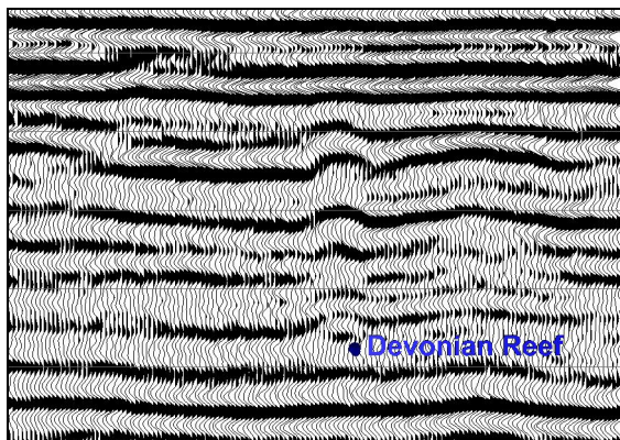
Figure 1.2: A conventional wiggle trace display of a small seismic section over a Devonian reef. Each wiggle represents the energy reflecting from a single common depth point. The deflection of the wiggle is proportional to the amplitude of signal. Positive amplitudes are displayed filled and to the right, negative amplitudes are displayed unfilled and to the left.
