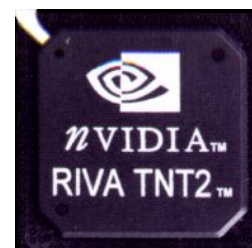
Figure 1.1: An NVIDIA RIVA TNT2 chip, one of the earliest graphic processing units.
