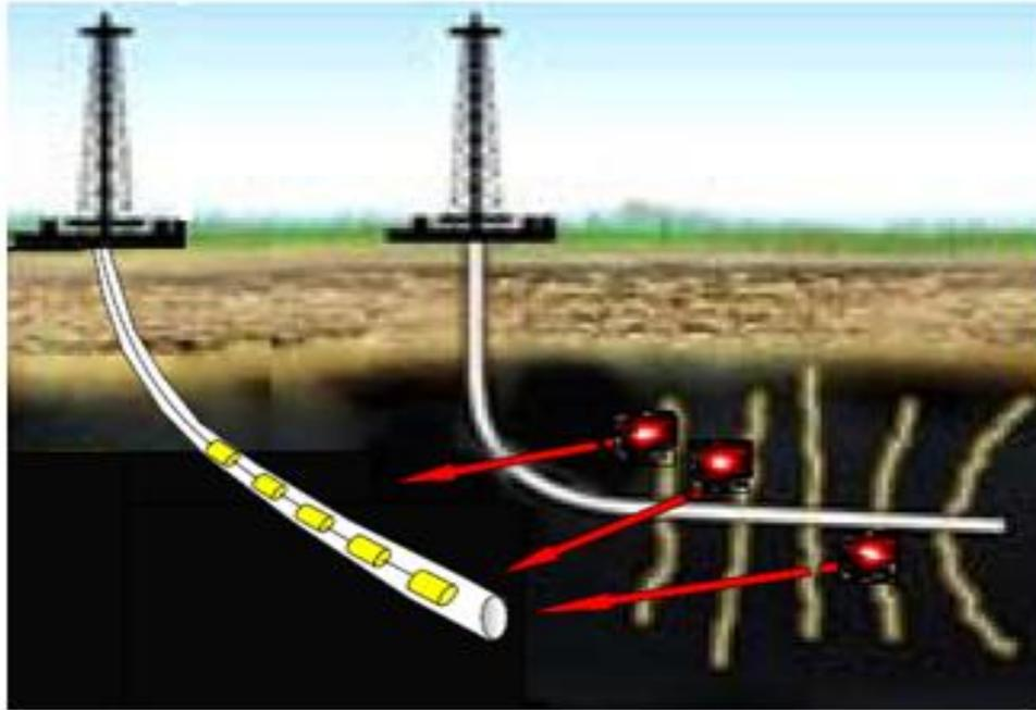
Figure 1.7: The observation well (left) monitoring microseisms with 3C geophones, and the treatment well (right) undergoing hydraulic fracture stimulation. (Courtesy Mahrer, 2009)
