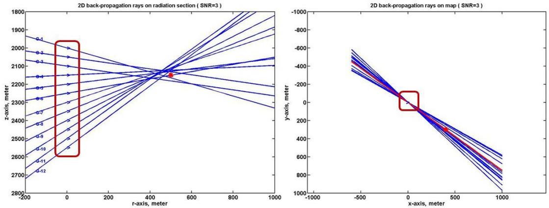
**Figure 5.5: The effectiveness of the 2D approach of hodogram analysis on noisy data. Resulted from synthetic data at SNR=3, the approximated propagations from the radial section (left) and the map (right) are less deviated from true propagations as shown in Figure 5.4(b).**
