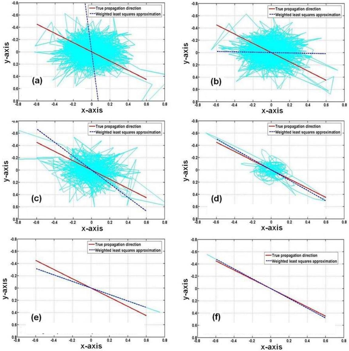
Figure 5.3: The hodogram linearity approximation using weighted least squares regression on (a) raw data and noise attenuation with (b) *bp*-filter, (c) *Mm*-stack, (d) *Mm*-stack and NSS, (e) *bp*-filter and NSS, and (f) *bp*-filter, *Mm*-stack, and NSS.
