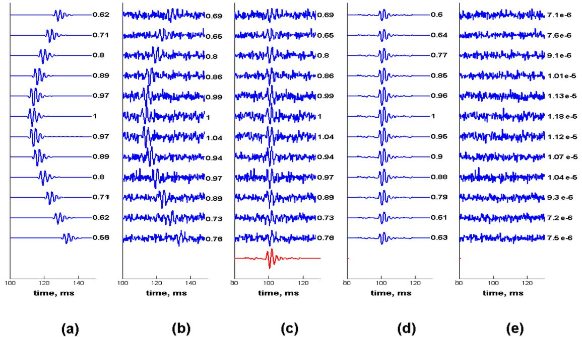
Figure 4.7: Noise attenuation and efficiency test. (a) seismograms of true waveforms; (b) noisy seismograms (c) noisy seismograms alignment after *bp*-filter and *Mm*-stack; the bottom red trace is the normalized stack trace; (d) signal component of noisy traces after NSS; (e) separated Gaussian noise components after NSS.
