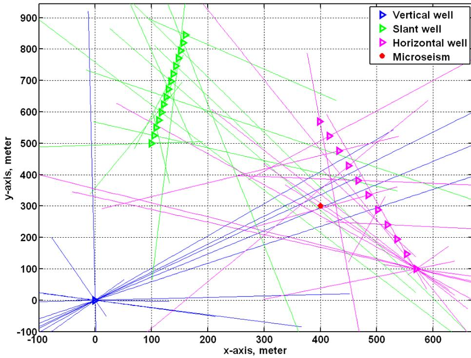
Figure A1.3: 3D and map views of raypaths of incident propagation derived on raw data from three wells.
