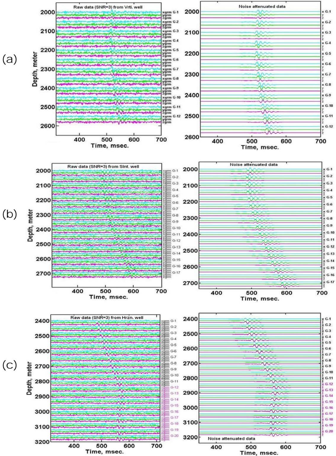
Figure 4.9: Noise attenuation (SNR effects) (the right column) on noisy 3C data (the left column) obtained from (a) a vertical well, (b) a slant well, and (c) a horizontal well, respectively at a SNR=3.
