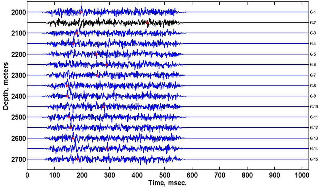
Figure 4.5: Inappropriate MER time picks on high noisy microseismograms ( $SNR \approx 1.3$ ).
