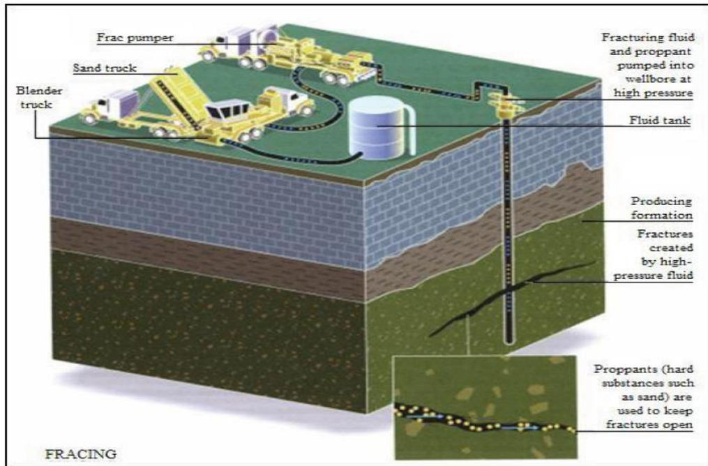
**Figure 1.6: Man-made rock fracturing in a hydrocarbon reservoir. Artificial rock fracturing increases the production in a well by injecting fluids/gas, sand, and a mixture of chemicals at high pressure and causing the formation rock to crack ([www.worc.org/userfiles/file/EPA-FracStudyFactSheet.pdf](http://www.worc.org/userfiles/file/EPA-FracStudyFactSheet.pdf)).**
