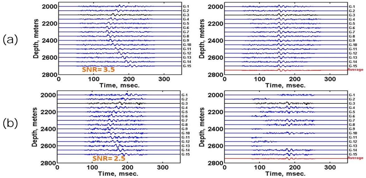
Figure 4.3: Noise limitation on the minimum variance technique with (a) containing traces with SNRs of 3.5 and (b) with SNRs of 2.5 he estimated alignments are shown on the right.
