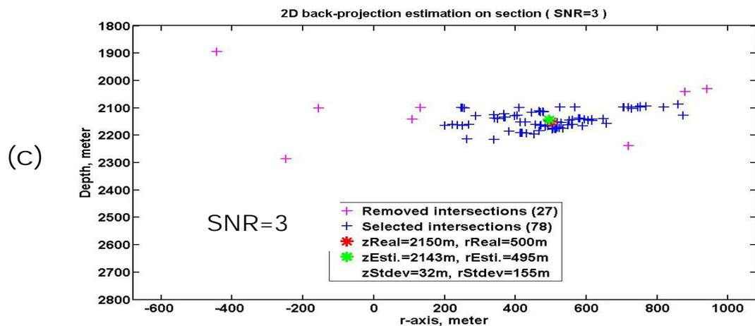
Figure 6.4: Statistical optimization on radial section. Clustering intersections (blue crosses) and outliers (pink crosses) are determined first, then the hypocenter estimate (the green star) to the true location (the red star) is located only from the clustering ones, at three noise levels as (a) SNR=2, (b) SNR=2.5, and (c) SNR=3.
