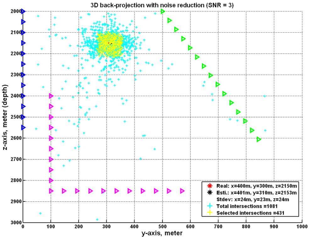
Figure A1.10: Section views of hypocenter location estimated on noise attenuated data from three wells.
