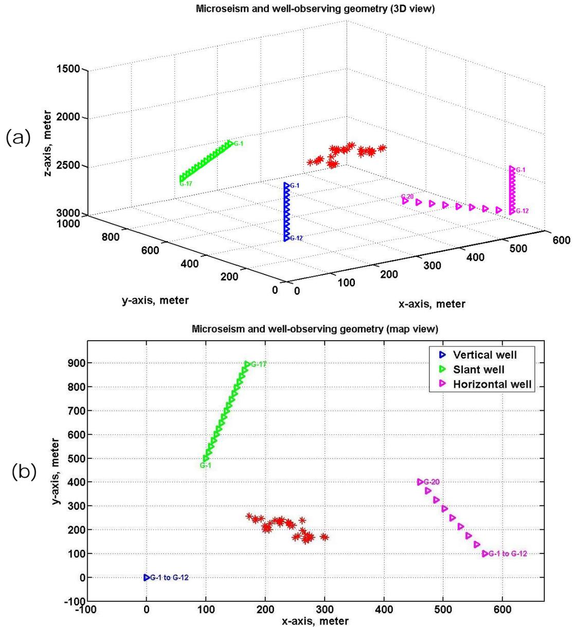
Figure 3.12: Multiple microseismic sources and the fracturing orientation.
