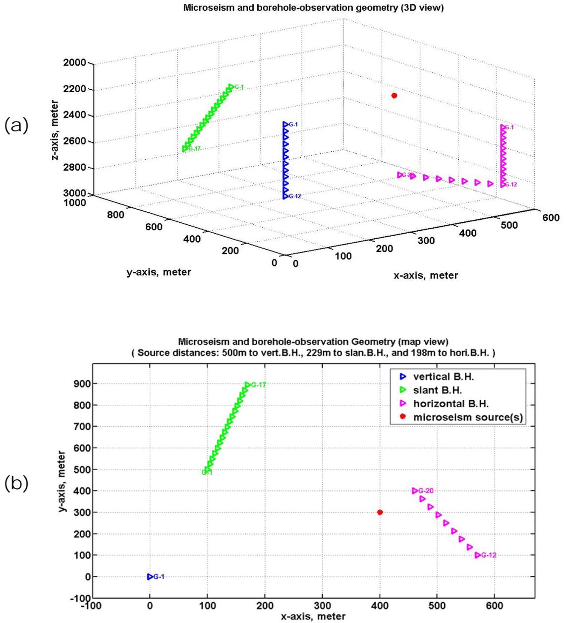
Figure 3.7: (a) The 3D geometry of multi-well monitoring of a single microseismic hypocenter, color-coded by the legend in (b) the map view.
