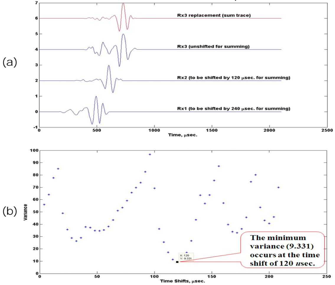
Figure 4.2: The minimum variance technique for trace shifting and stacking. Three traces (Rx1, Rx2, and Rx3) are shown in (a) the optimal shift  $\Delta t = 120 \mu\text{s}$  corresponding to the minimum variance (9.331) is found through a series of calculation of (shift, variance) pairs in (b).
