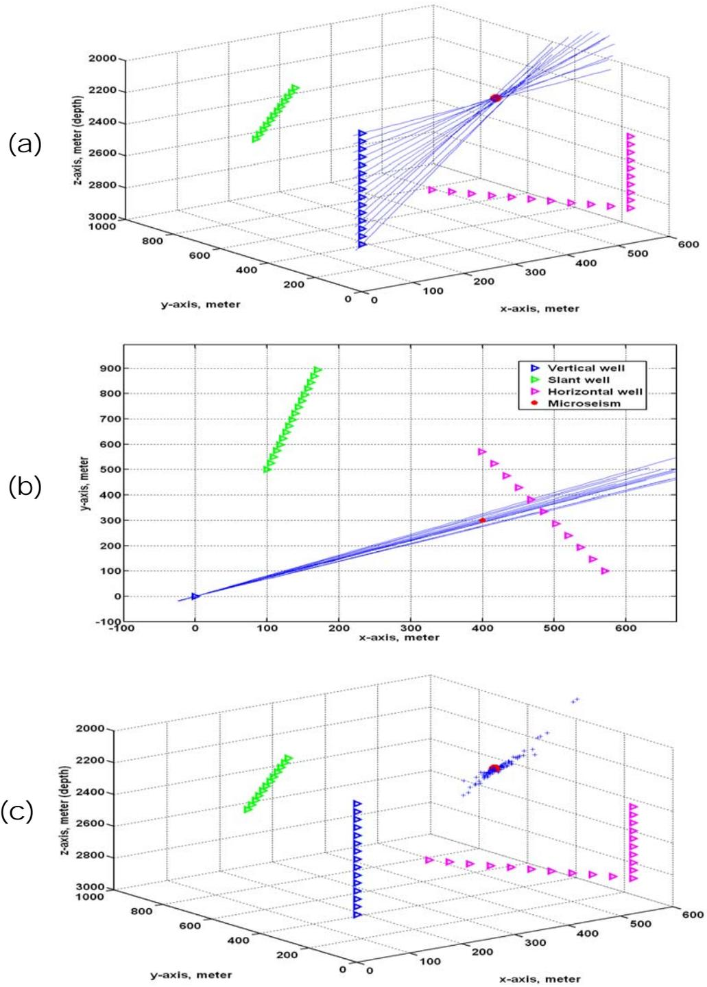
Figure 6.1: Illustration of the 2D approach of back-propagation analysis (in 3D view). It is based on (a) propagations (blue lines) in a vertical array of 3C geophones (blue triangles) to a single microseism (red dot), (b) the map projection of propagation raypaths, and (c) nearest points (blue crosses) of mutual raypaths to be projected on the radial section. The well is shown in a 3D volume with receivers in other wells (non-blue triangles) that are not used.
