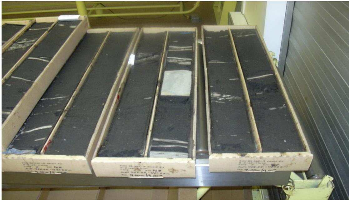
Figure 3. 10 Cores of reservoir rock (oil sands)
