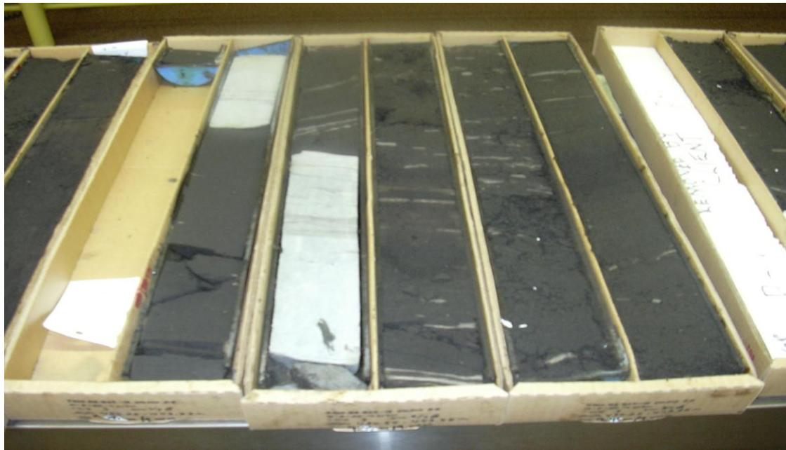
Figure 3. 8 Cores of reservoir rock (oil sands)
