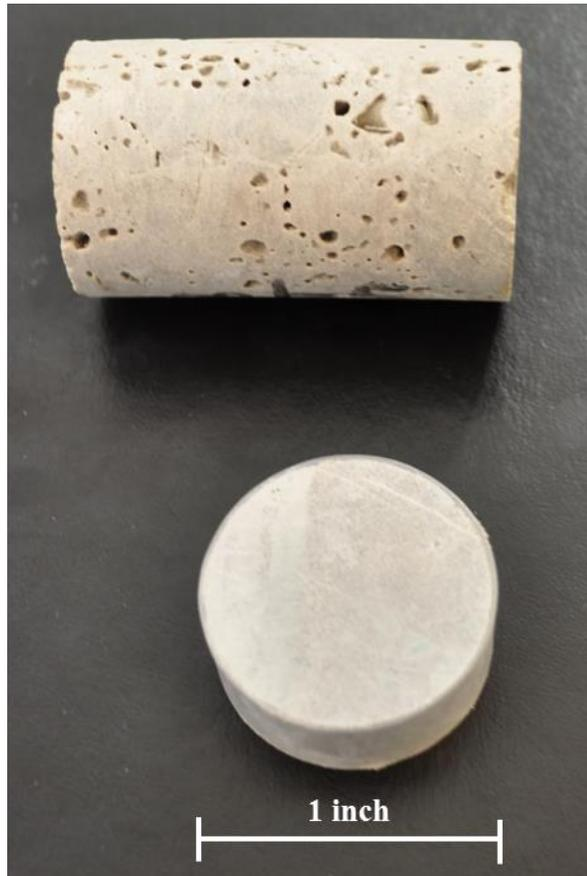
**Figure 3.20: Nisku core sample and Calmar core plug recovered from Well 8-17 during the development of Project Pioneer. Diameter = 1 inch (modified from Carbon Management Canada, 2013: <http://www.cmc-nce.ca/events/gallery/>).**
