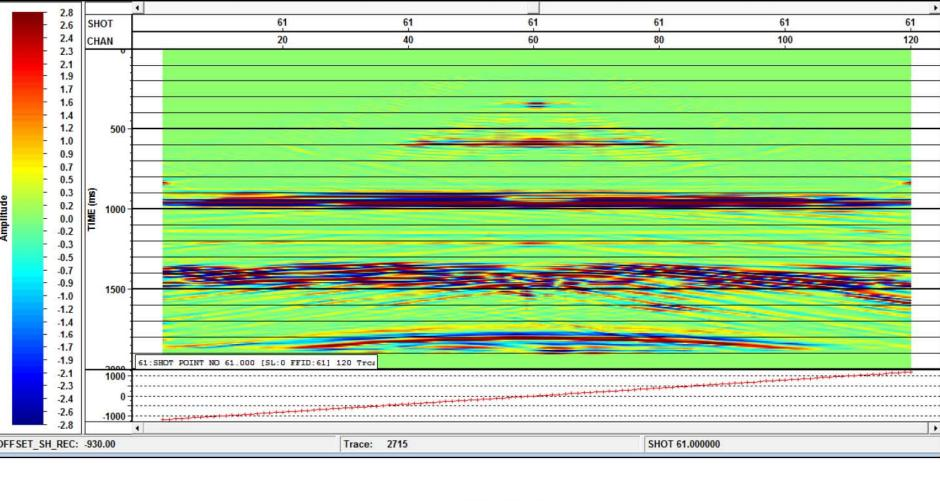
This is shot record 61, which has been NMO corrected. There are three primary events that can be seen, The first two are gradient changes at 0.35s and 0.6s and the channel interval at about 0.9s. There is also some converted wave response at 1.4s and shear response at 1.8s.
