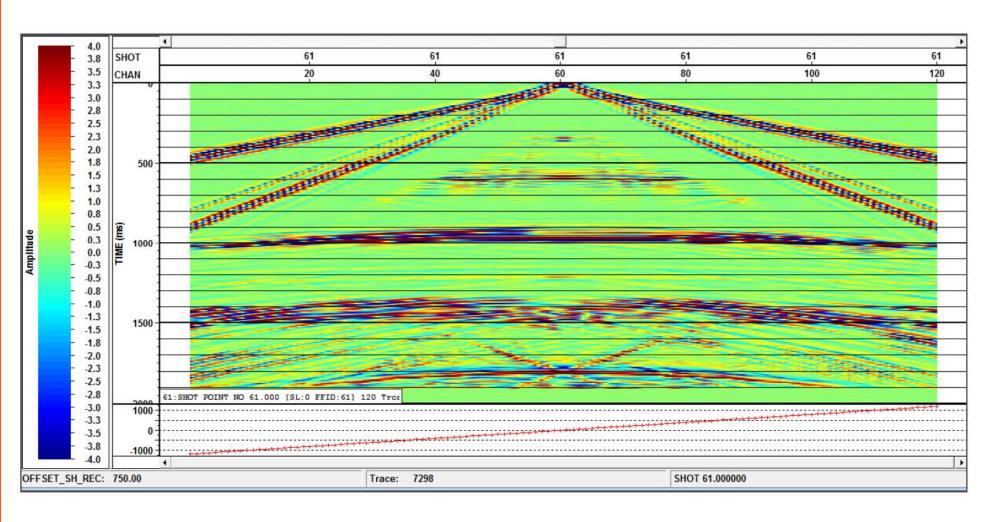
This shot record has an AGC and a scaling function applied. It has also had a bulk time shift of 0.1 seconds applied to correct for the time shift that is present in the wavelet.
