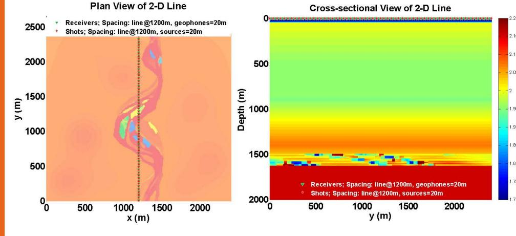
The figure on the far left shows the geometry and position of the 2-D line used in this flow. The other figure shows the Vp/Vs ratio from the velocity model along with the geometry of the line indicated at the top of the figure.
