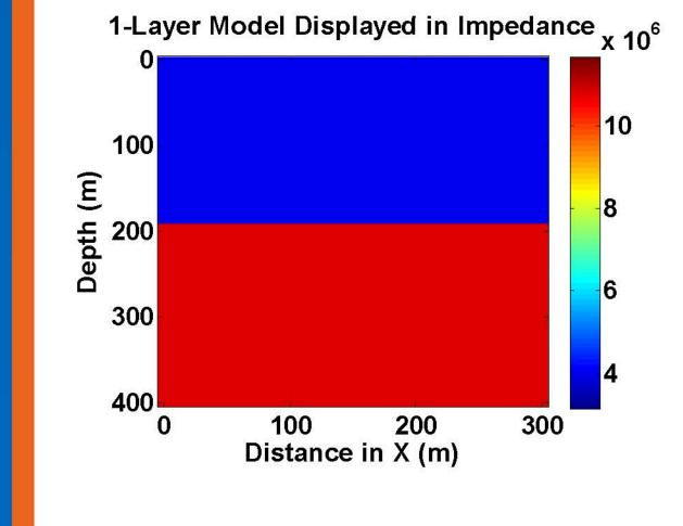
To determine the polarity of the data, a test was done with a one layer model where the lower layer of the model has higher impedance. It can clearly be seen from the data collected that the response of a positive impedance contrast is a peak to the right.
