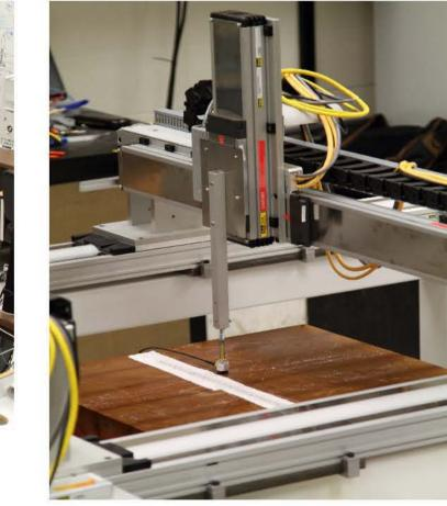
► **Source and receivers:** These are flat-faced piezoelectric cylindrical transducers with the diameter of 13*mm* and central frequency of 1.0*MHZ*.
