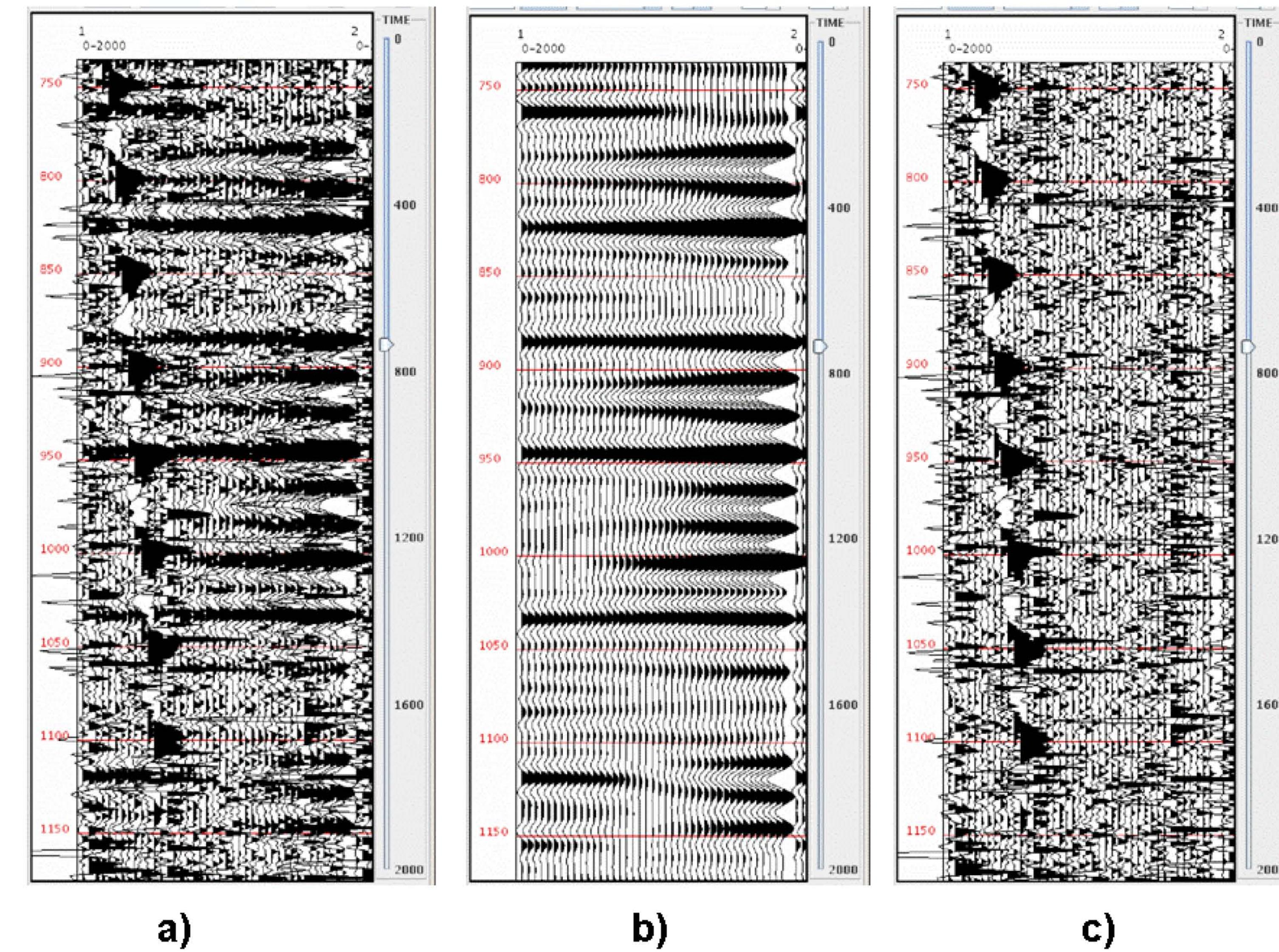
FIG. 2. Synthetic CDP gather with noise a), CDP gather after noise attenuation b), removed noise c).
