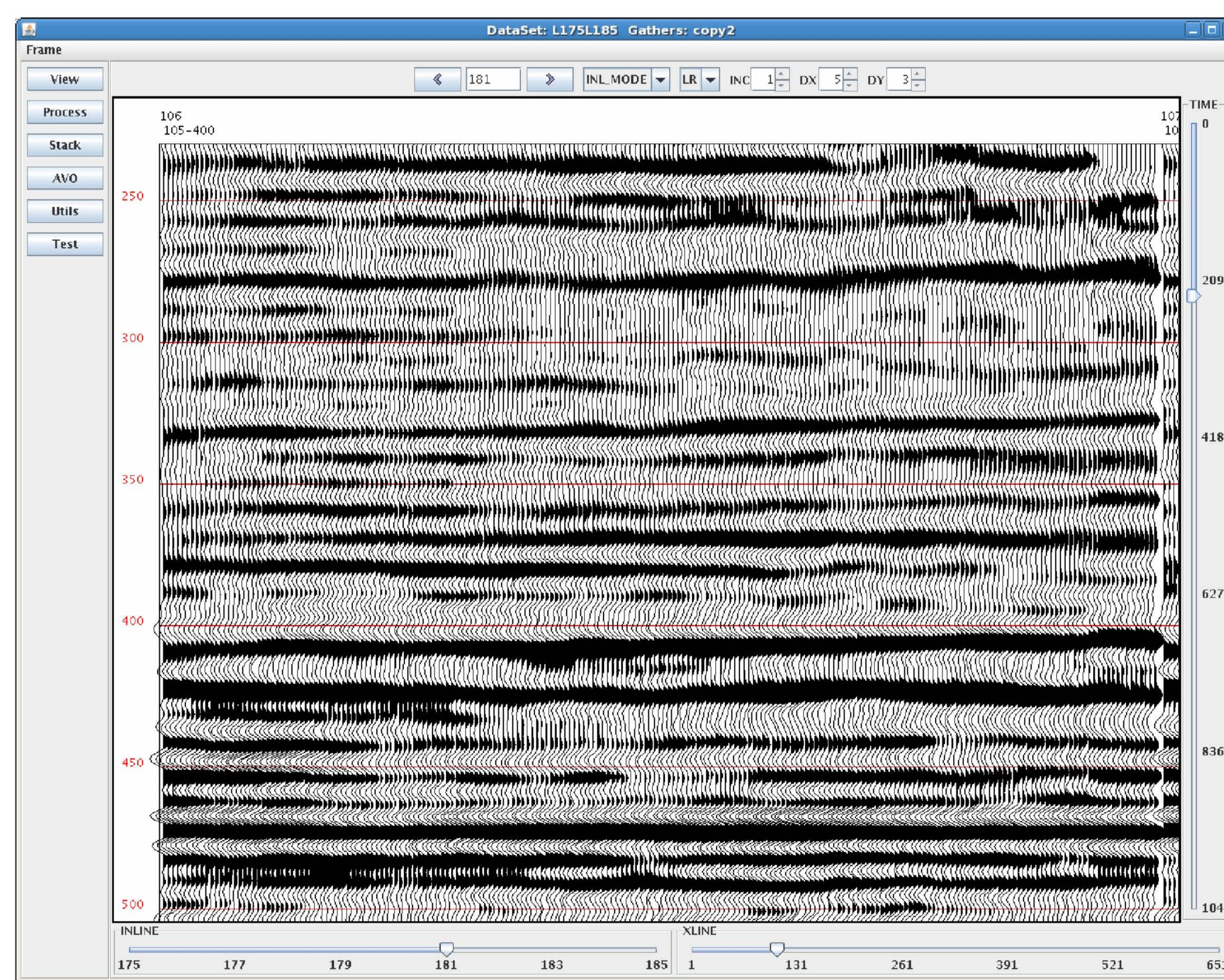
FIG. 4. Alberta oil sands CDP gather after local linear models noise attenuation. Both, the low frequency and random noise have been removed successfully.
