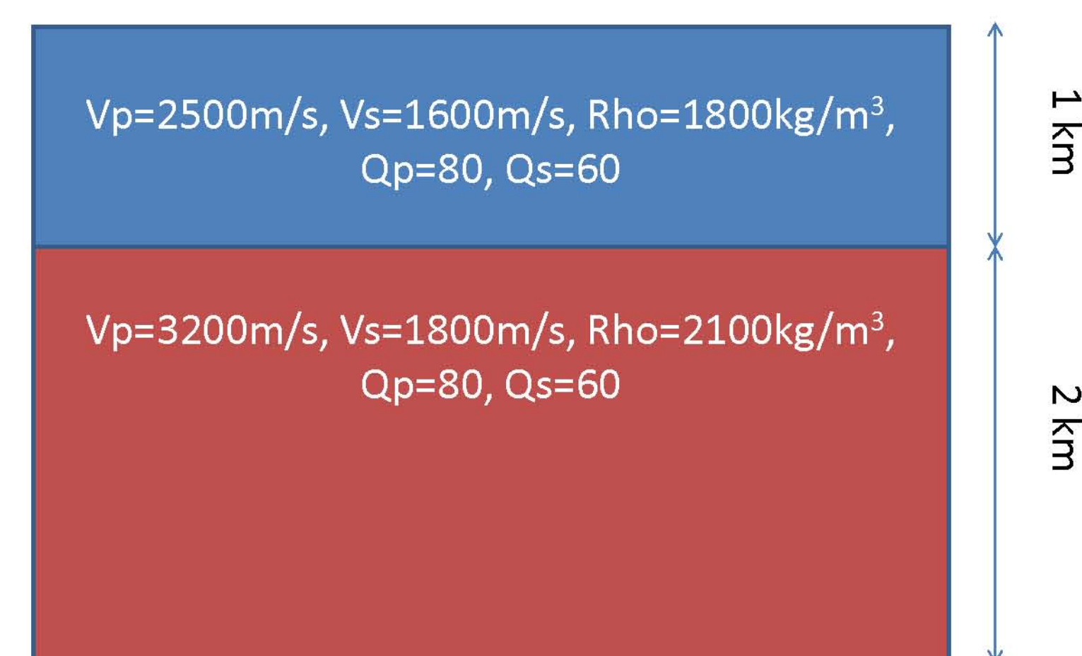
FIG. 2. A two layer earth model with attenuation.
