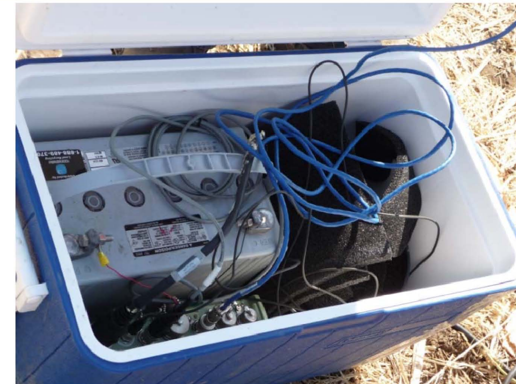
FIG. 2. Car battery and Taurus recorder inside a food cooler
