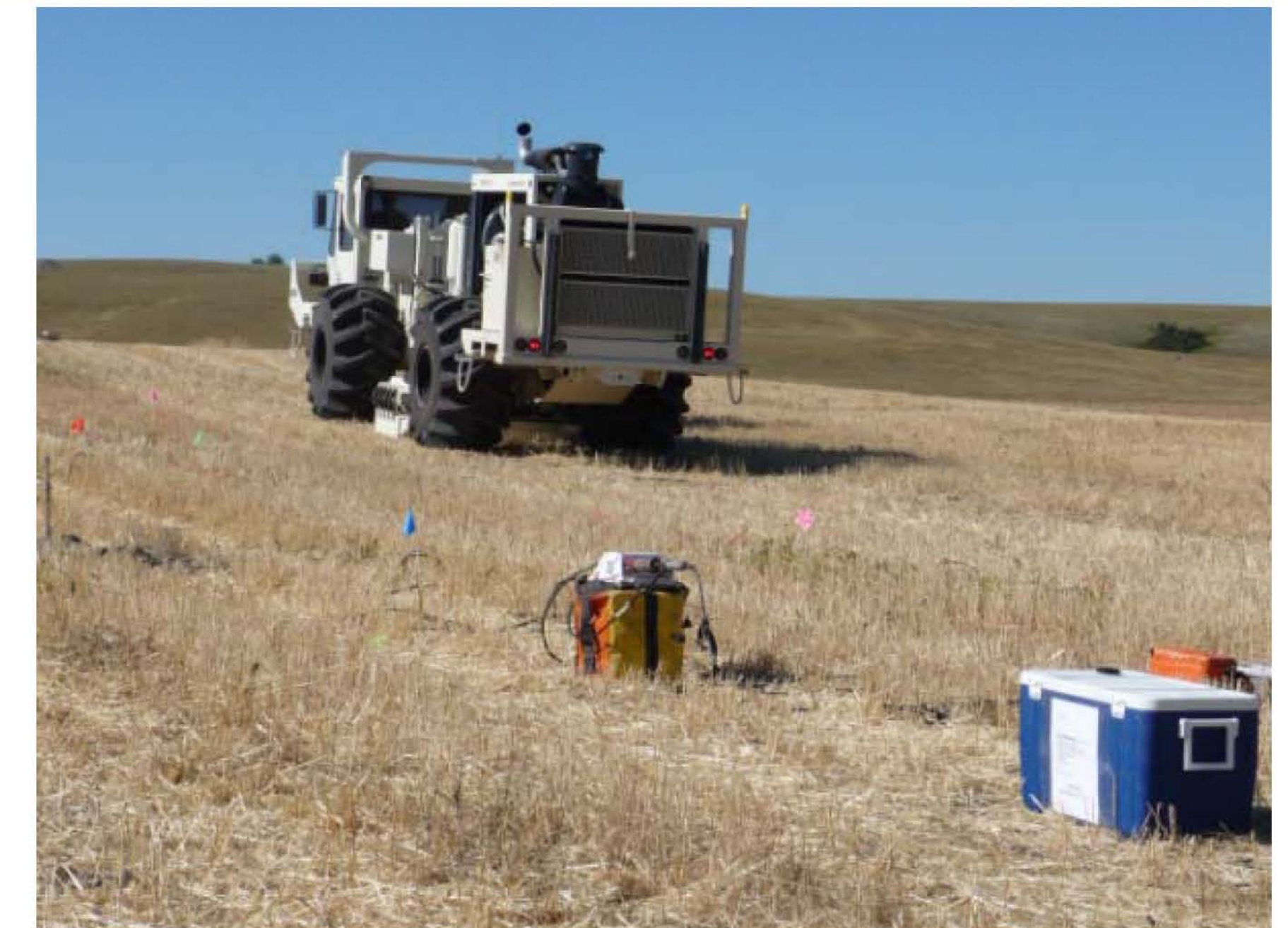
FIG. 3. Cooler on the ground near VectorSeis and Aries equipment, during an INOVA 364 low-frequency vibe sweep (right).
