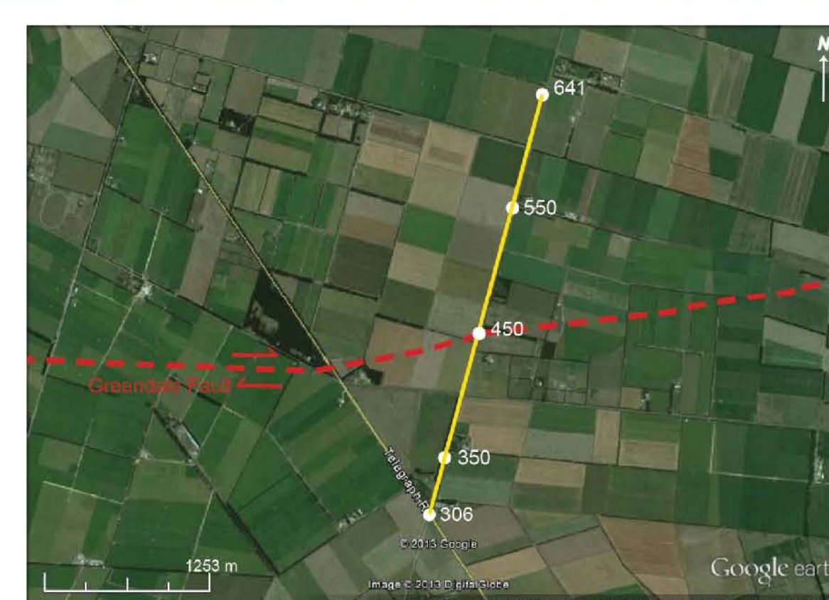
Fig 3b. Highfield Road seismic line (in yellow). Started on south end at station 306 and ended north at station 641. The Greendale Fault ruptures the surface in an E-W orientation. Google earth V 7.0.3.8542. (28 January 2013) Highfield Road, New Zealand.
