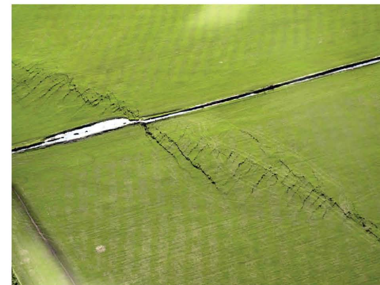
Fig 2b. Aerial photograph of the E-W trending Greendale Fault. A drainage canal is displaced by shear fractures along the fault surface. Image taken by Richard Jongens of GNS science.
