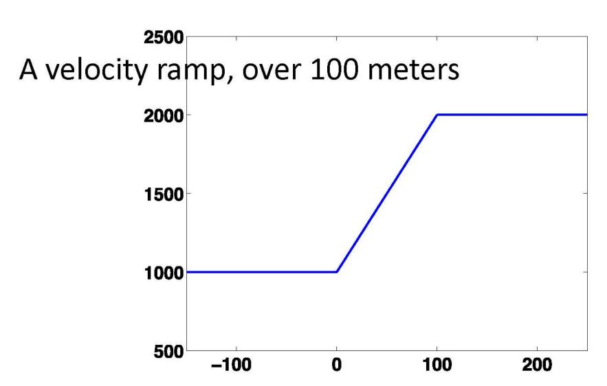
Wave propagation through the transition zone, constant bulk modulus
