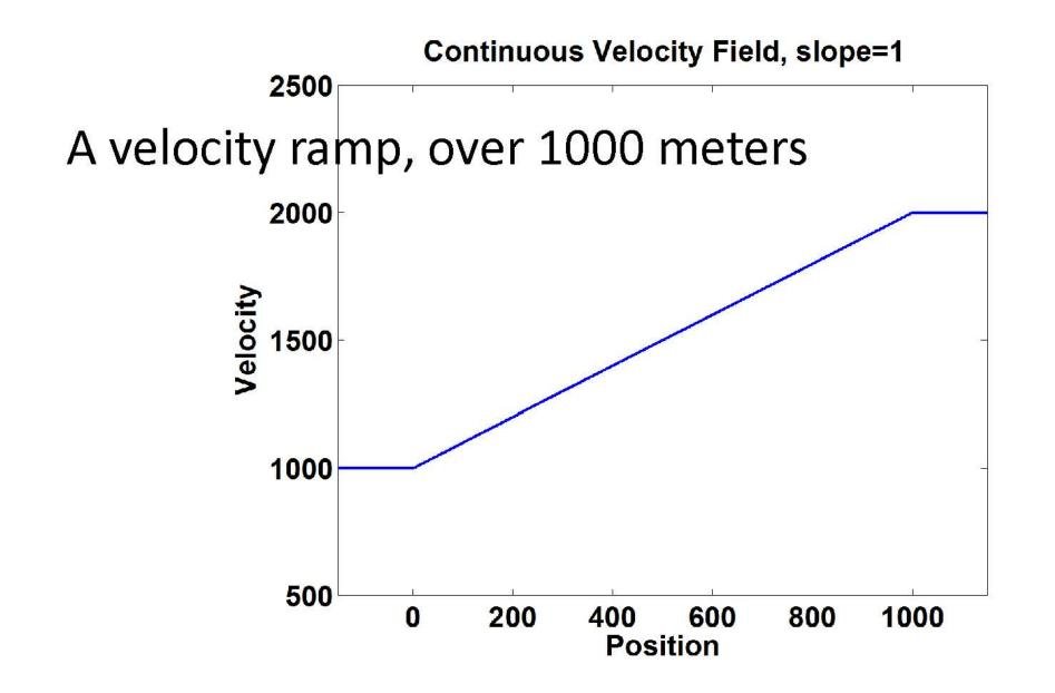
Beginning with a 1D elastic wave equation, we can produce exact analytic solutions for waves propagation through the velocity ramp. By applying continuity conditions at the interface, we compute the frequency dependent reflection and transmission coefficients
