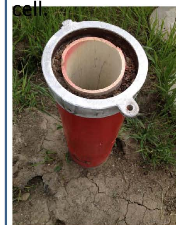
FIG 1. Well 4 before the installation of the coil tubing. The bentonite grout between the PVC casing and the steel conductor casing is visible. The ID of the PVC restricted the size of coil tubing that could be inserted to 2.875 inches, resulting in an available ID of approximately 2.5 inches. This allows for a 2 inch diameter probe to fit alongside a 0.25 inch tube for gas bubble insertion.
