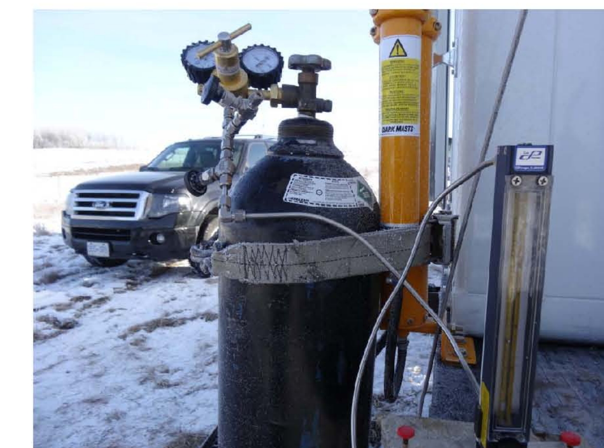
FIG 10. The nitrogen bottle and flow meter / regulator used for this test.
