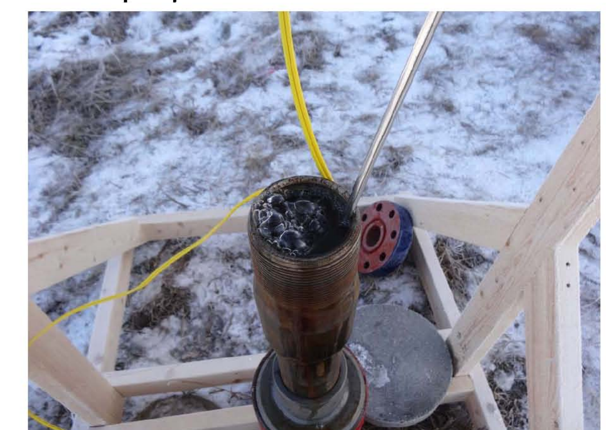
FIG 11. Bubbles coming to surface in the coil tubing.
