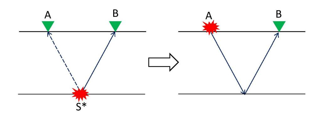
Convolution of events with the same rayparameter value returns events with larger traveltime. The figure shows how reflection times can be computed from one way times.
