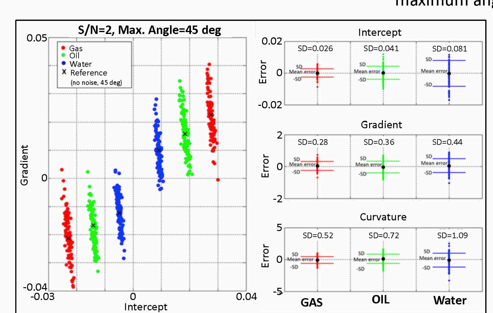
FIG. 8. Calculating the standard deviation (SD) of 100 estimations for S/N=2 and Max. Angle=45 deg. The SD represents the uncertainty of the AVO-parameter estimation.
