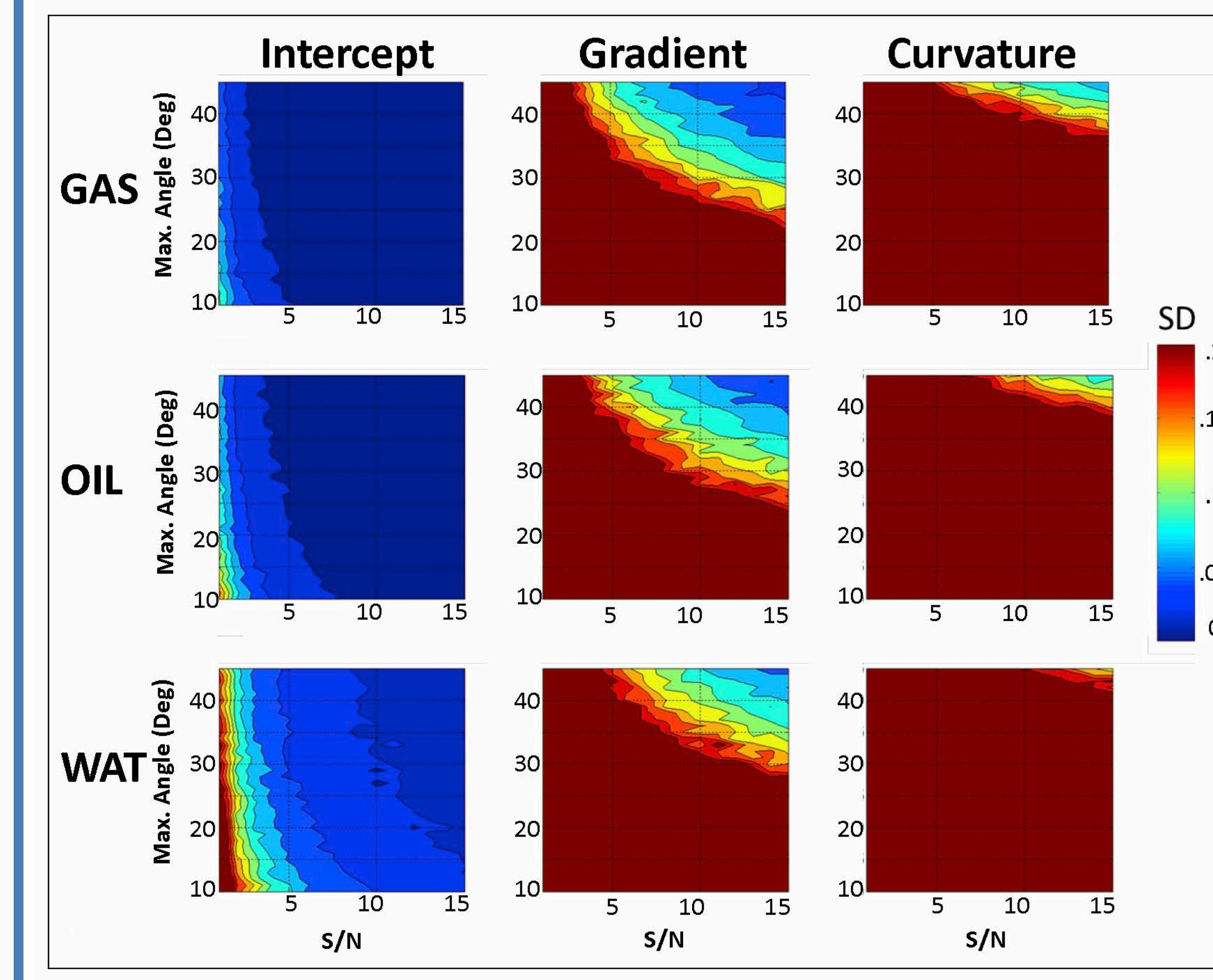
FIG. 9. Simultaneous effect of noise and maximum angle available on AVO-parameter estimation.
