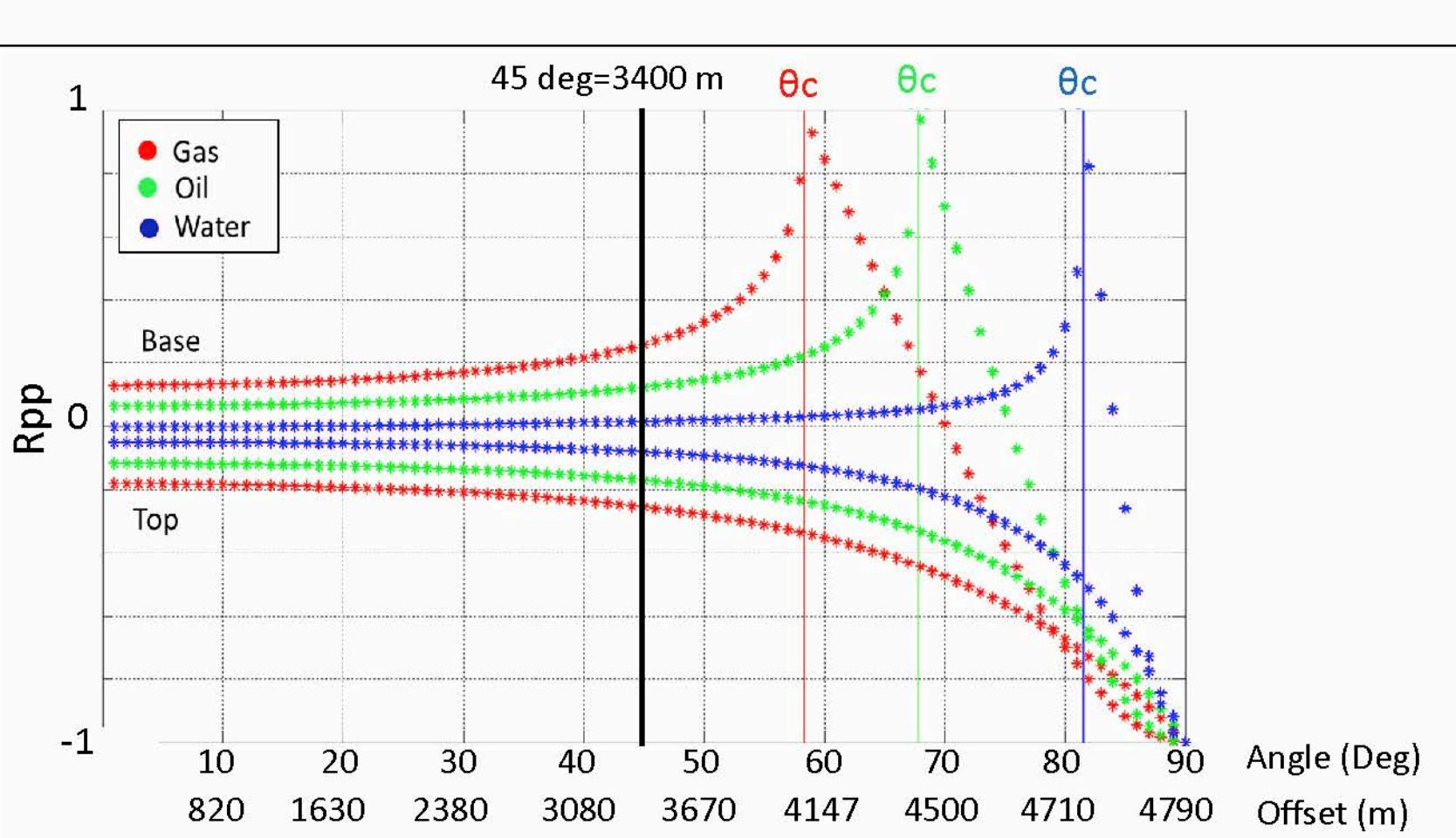
FIG. 2. Reflection coefficient variation with angle of incidence (or offset) for the three fluid scenarios. Pre-critical angles smaller than 45 degrees were used in this experiment
