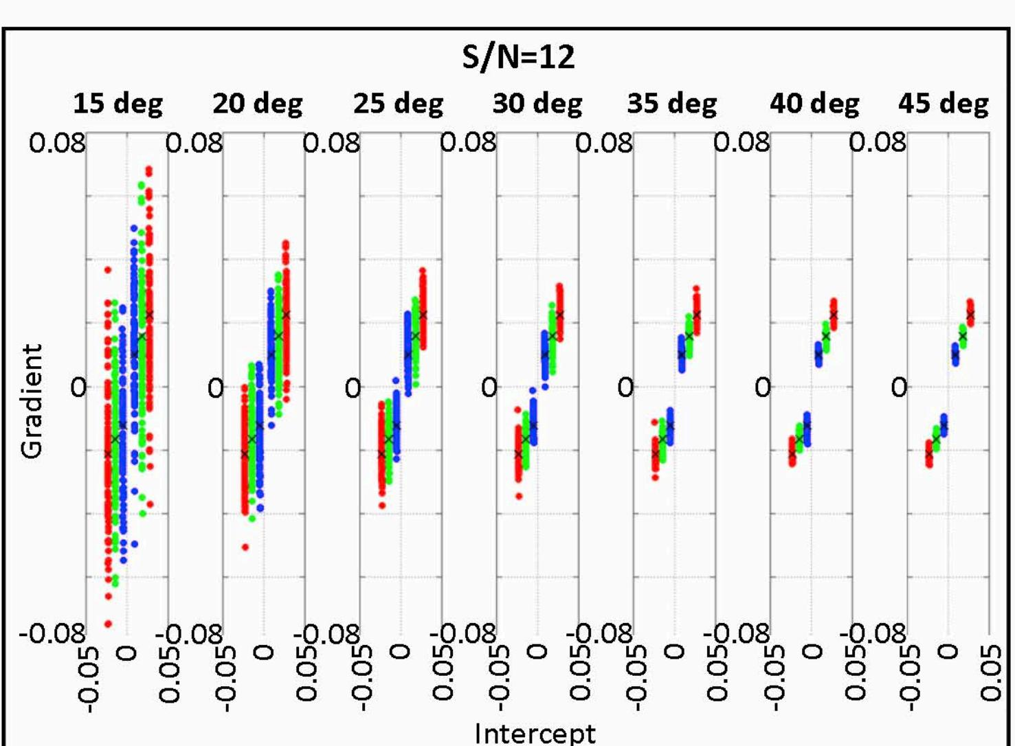
FIG. 7. Dispersion of the AVO-parameter estimation produced by the reduction of the maximum angle available.
