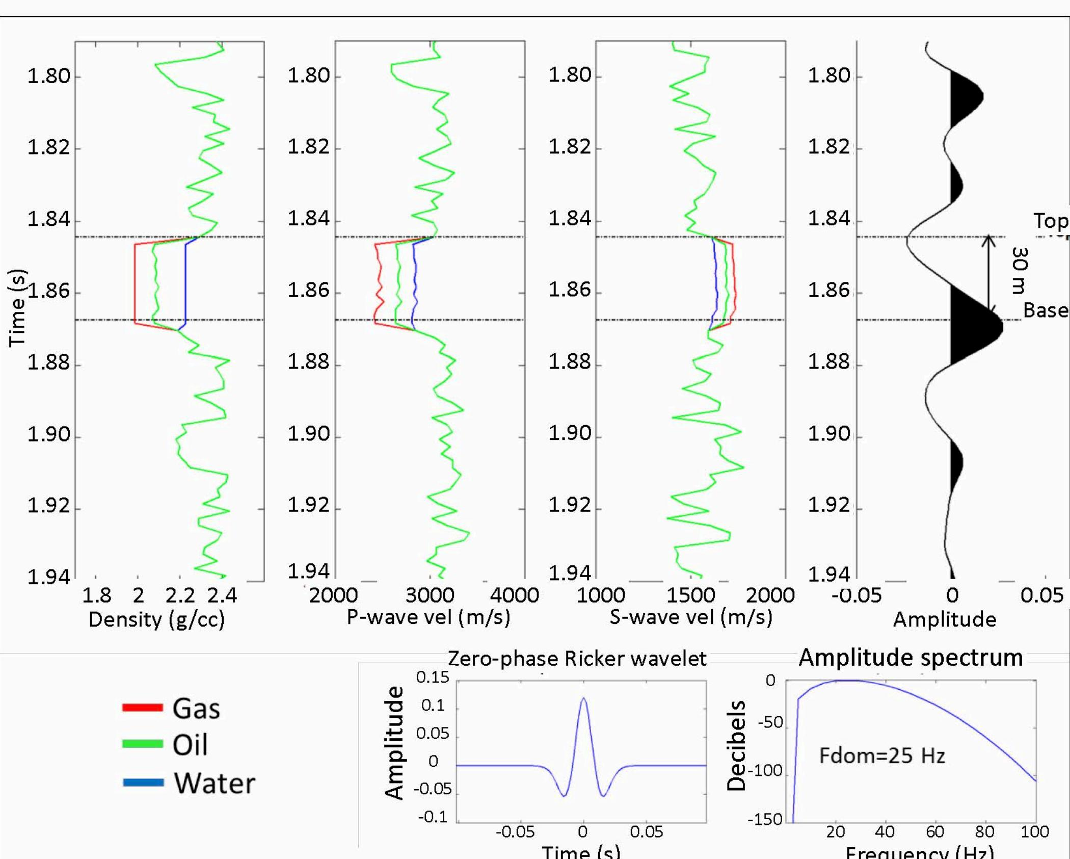
FIG. 1. Well log data of an oil-producing well. The original logs (green) correspond to oil filling the pore space. The red and blue lines correspond to gas and water, respectively. A zero-phase Ricker wavelet with dominant frequency of 25 Hz properly resolves the reservoir.
