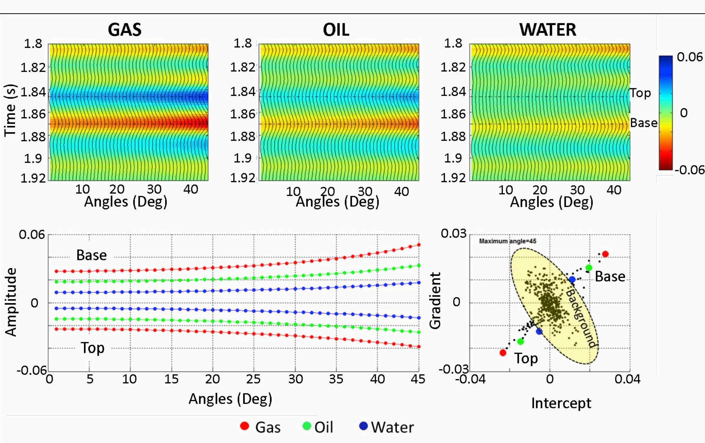
FIG. 3. Synthetic seismic gathers with AVO response for gas, oil and water sands. The intercept and gradient parameters are derived by fitting equation 1 to the amplitude vs angle points. The intercept vs gradient plot discriminates fluids.
