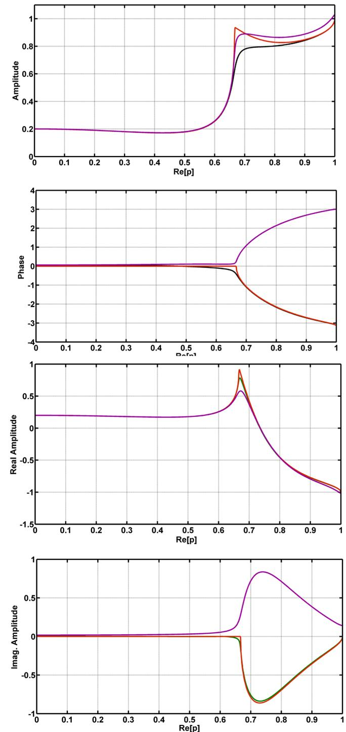
Fig.3.  $P_1P_1$  reflection coefficient. The upper two panels show the amplitude and phase plotted versus the real value of horizontal slowness. The bottom two panels show the real and imaginary parts plotted versus the same quantity. Red indicates the reference elastic case. Purple indicates the anomalous case before corrections.
