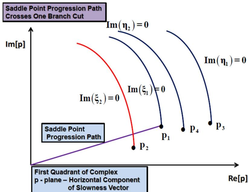
Fig.2. A schematic of the first quadrant of the complex  $p$ -plane (horizontal component of the slowness vector). The *saddle point progression path* is the values that the incident  $P$ -wave may have corresponding to the elastic case of  $[0 \leq \sin \theta / \alpha_1 \leq 1; 0 \leq \theta \leq \pi/2]$
