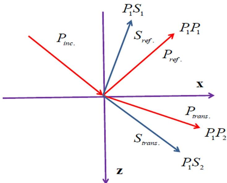
Fig.1. A schematic of a  $P$ -wave incident from the upper medium on an interface between two media and the resulting wave types that arise. The subscripts "inc.", "ref." and "trans." refer to incident, reflected and transmitted modes, respectively.
