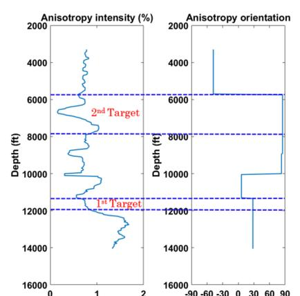
S-wave analysis: anisotropy intensity (left) and direction (right).
