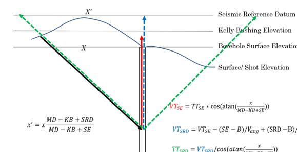
A schematic diagram showing borehole and downgoing raypath from shot to geophone, indicated by black arrow. X is the borehole-shot offset. Vertical raypath from shot elevation is indicated by red arrow. Blue arrow indicates vertical raypath to SRD. The shot to geophone traveltime is calculated from SDR and indicated by green arrow.
