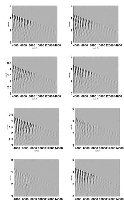
4-C VSP before rotation: N-S shot components (top), E-W shot components (bottom), N-S receiver components (left), and E-W receiver components (right).
