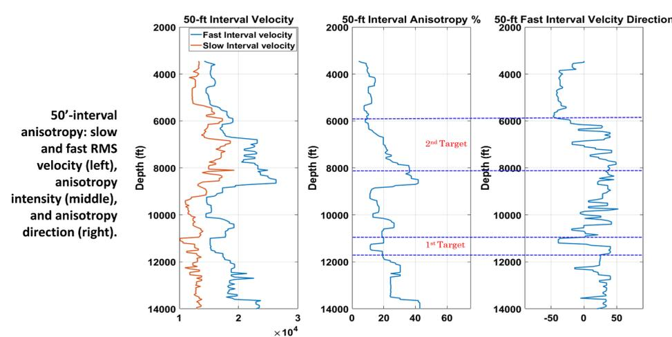
50'-interval anisotropy: slow and fast RMS velocity (left), anisotropy intensity (middle), and anisotropy direction (right).
