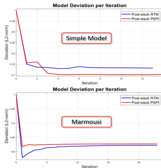
Normalized model deviation (L2-norm) of the PSPI (red line) and RTM (blue line) migrations. The choice of which migration to use will depend on the complexity of the geology and computational resources.
