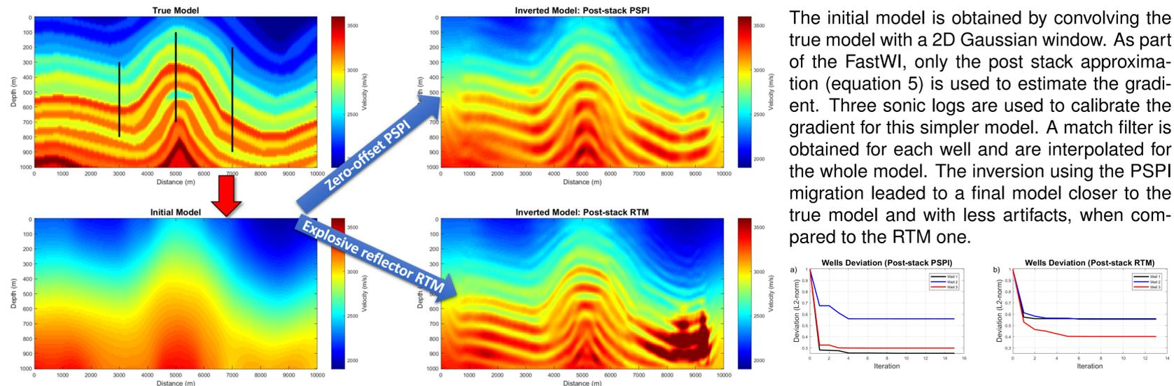
The initial model is obtained by convolving the true model with a 2D Gaussian window. As part of the FastWI, only the post stack approximation (equation 5) is used to estimate the gradient. Three sonic logs are used to calibrate the gradient for this simpler model. A match filter is obtained for each well and are interpolated for the whole model. The inversion using the PSPI migration led to a final model closer to the true model and with less artifacts, when compared to the RTM one.
