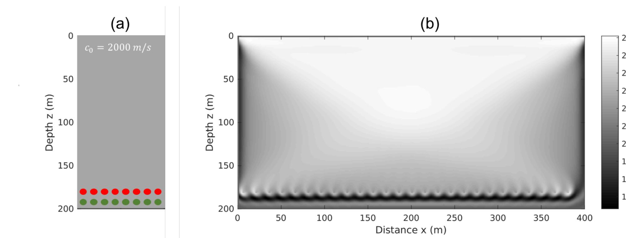
Figure 5: Moving the sources gives a bulk update to the model.
