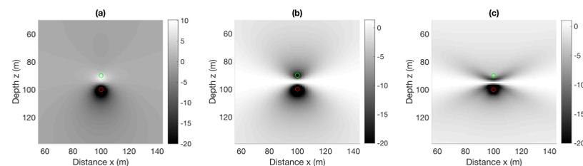
Figure 4: Gradient as a function of frequency: (a) 5 Hz, (b) 20 Hz, (c) 40 Hz.
