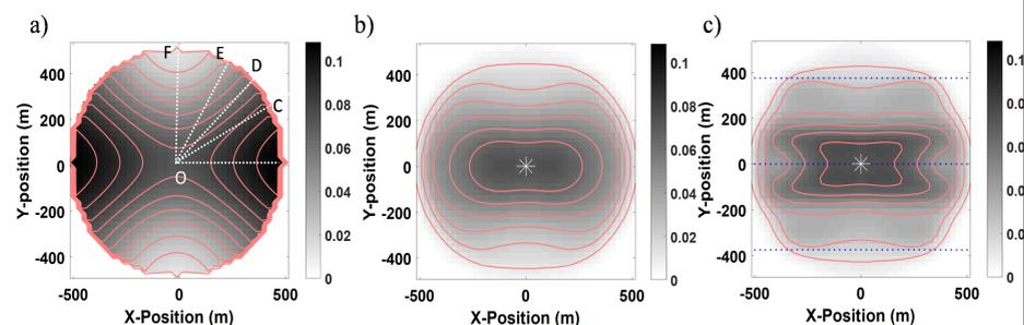
Fig.2. Evaluation of radiation patterns for an anisotropic HTI model. a) Analytical evaluation. b) Well-sampled Kirchhoff modeled data and c) the poorly-sampled modeled data.
