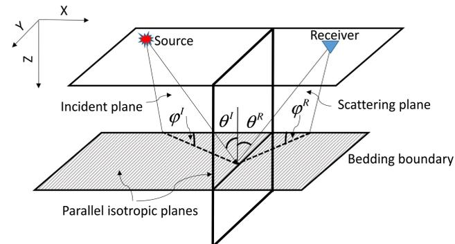
Fig.1. Schematic representation of reflection in transversely isotropic medium.
