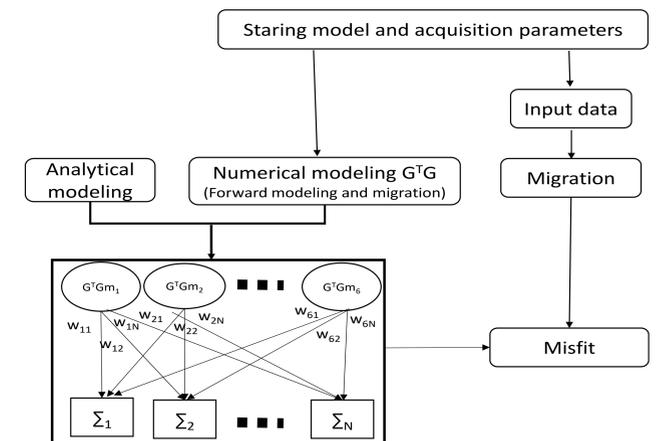
Fig.4. Flow work for AVO/Az analysis using basis dictionaries and constrained solution.
