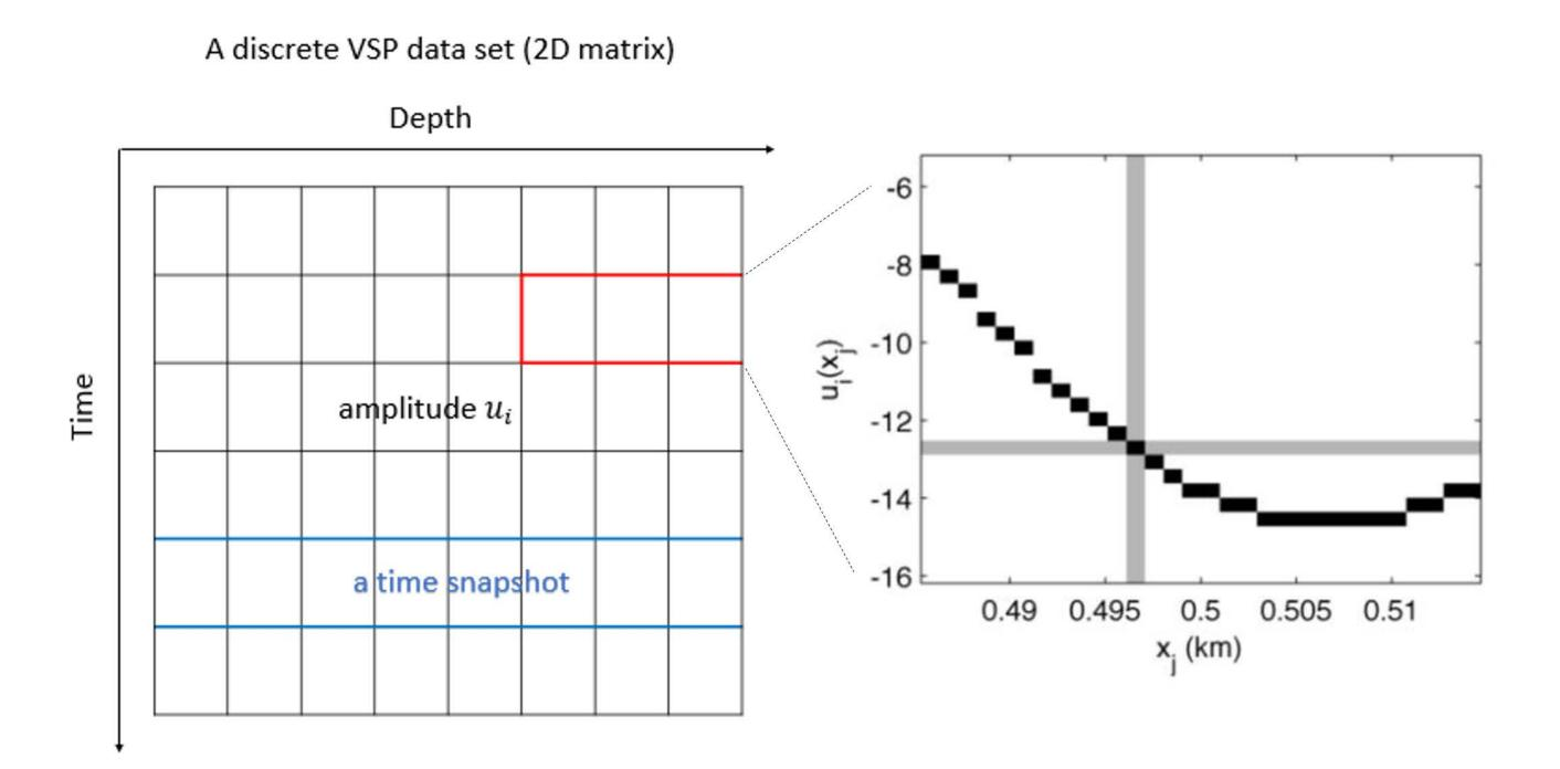
For a discrete VSP data set, assume each of its time snapshots to be a "message", and data points with amplitude  $u_i$  in the snapshot can be regarded as the "letters" which make up the "message".
