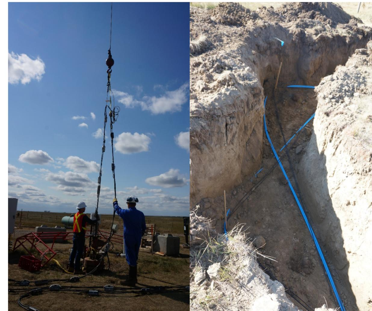
Left: 324 1Hz vectorseis receivers being put down the observation well.
