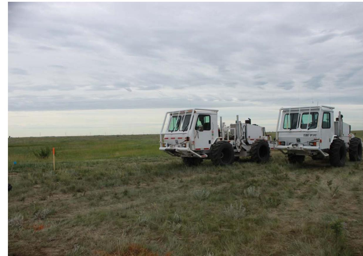
Echo Seismic Ltd.'s S-wave Envirovibe and the Seismic Group's Envirovibe.
