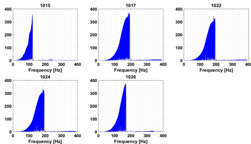
FIG. 3: Amplitude spectra for pilot trace (nearest geophone) for five test sweeps of GPUSA borehole linear vibrator.
