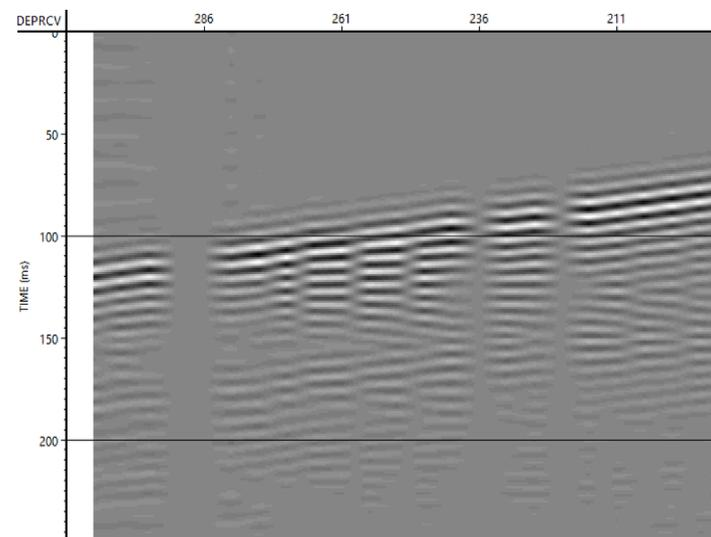
FIG. 4: Raw VSP data from borehole linear vibrator source. Data correlated with surface geophone nearest source location. Sweep is 0-175 Hz for 25 sec. Symmetric down-sweep.
