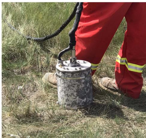
FIG. 2: GPUSA borehole linear vibrator prior to installation. Rotation axis for this source is vertical.
