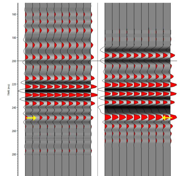
FIG. 6: Corridor stacks for borehole linear vibrator (left) and Vibroseis (right) VSP data. Injection interval highlighted by arrows.
