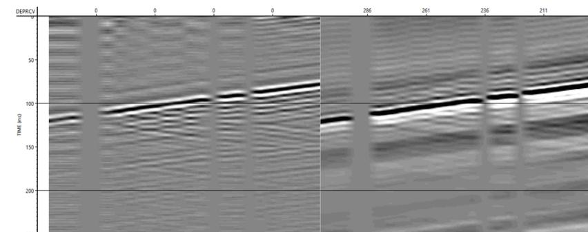
FIG. 5: VSP data from borehole linear vibrator (left) and Vibroseis (right) with Gabor deconvolution applied.
