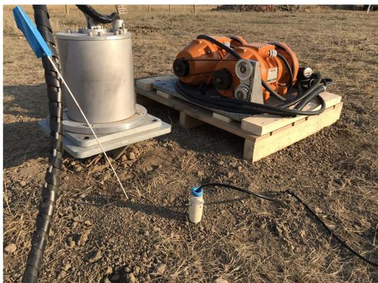
FIG. 1: GPUSA surface linear vibrators with geophone for scale. Rotation axes for these sources are horizontal.
