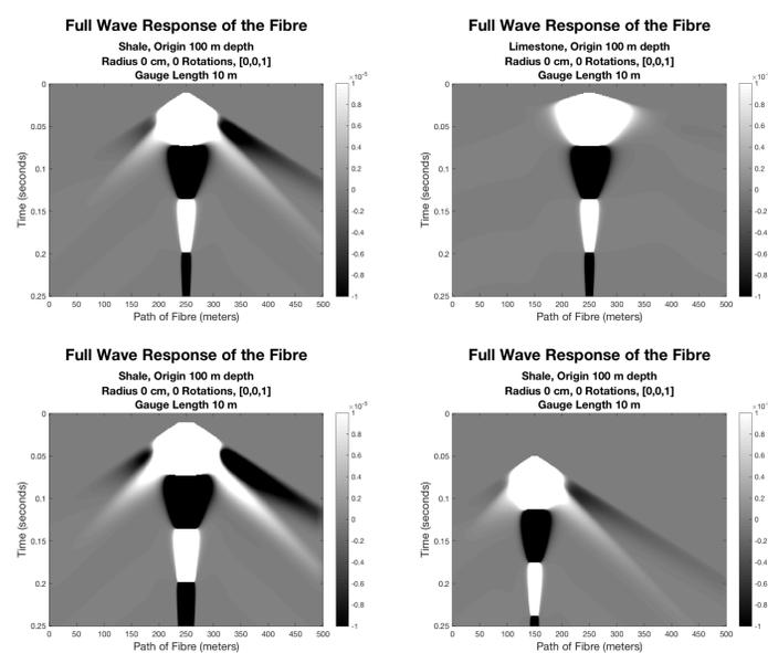
Figure: Synthetic examples of (Top row) signals from seismic waves moving at two different velocities. (Left column) signals acquired using two different gauge lengths. (Bottom right) signal from a shifted source location.
