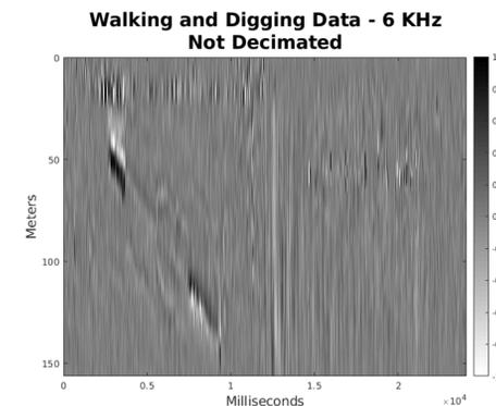
Figure: The 6kHz PRF data set which has not been decimated of someone walking next to the fibre and someone digging next to the fibre.
