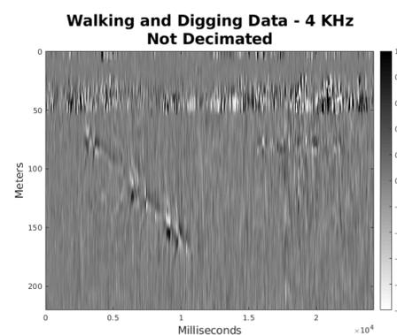
Figure: The 4kHz PRF data set which has not been decimated of someone walking next to the fibre and someone digging next to the fibre.
