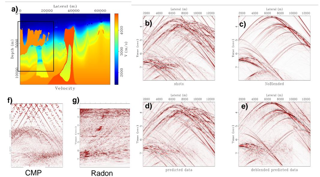
Example of deblending by inversion in a difficult data set. Although a hyperbolic Radon transform was used for all these examples, a more flexible transform may be necessary in complex cases. a) velocity, b) 5x supershot (blended), c) never-blended shot d) result of data fitting e) deblended shot, f) A pseudo-deblended CMP, g) Radon transform subpanel of f).
