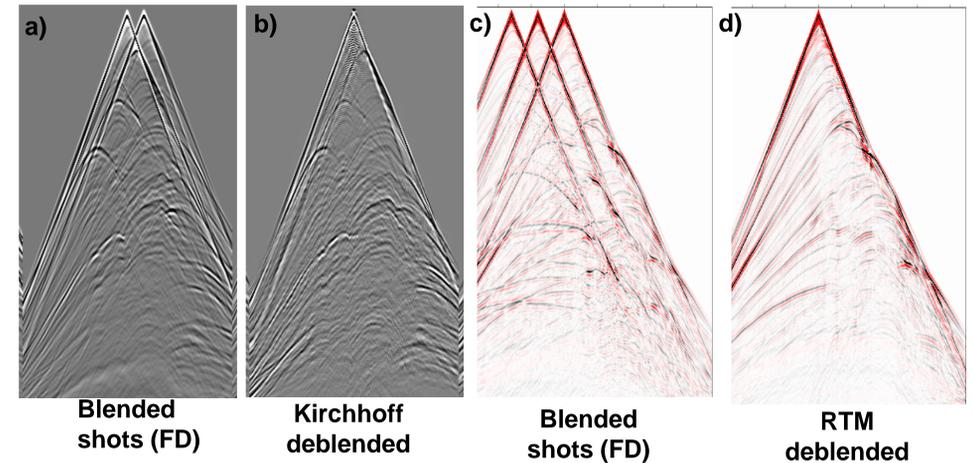
**Physical transforms:** use physics to map the blended data to the subsurface physical model. Once the model is built, shots can be predicted in the deblended (extended) space. a) 2x supershot b) deblended by Kirchhoff depth migration, c) 3xsupershot, d) deblended by RTM
