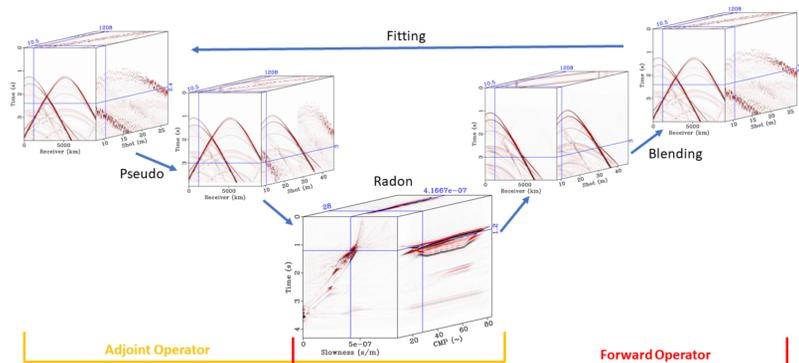
Figure 2: Illustration of the Blending operator. Where the unblended source is blended using the blending operator to output the blended data set.
