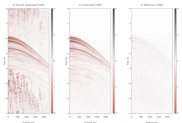
Figure 6: Gulf of Mexico data in CMP domain: Deblending using a gulf of Mexico marine dataset with results in the CMP domain, with Blended data in a), deblended in b), and difference in c).
