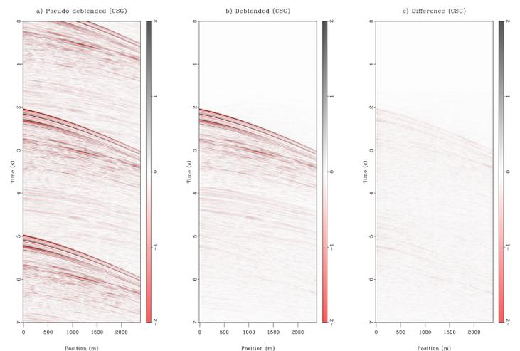
Figure 5: Gulf of Mexico data: Deblending using a gulf of Mexico marine dataset with an shot time interference of 70%, with Blended data in a), deblended in b), and difference in c).
