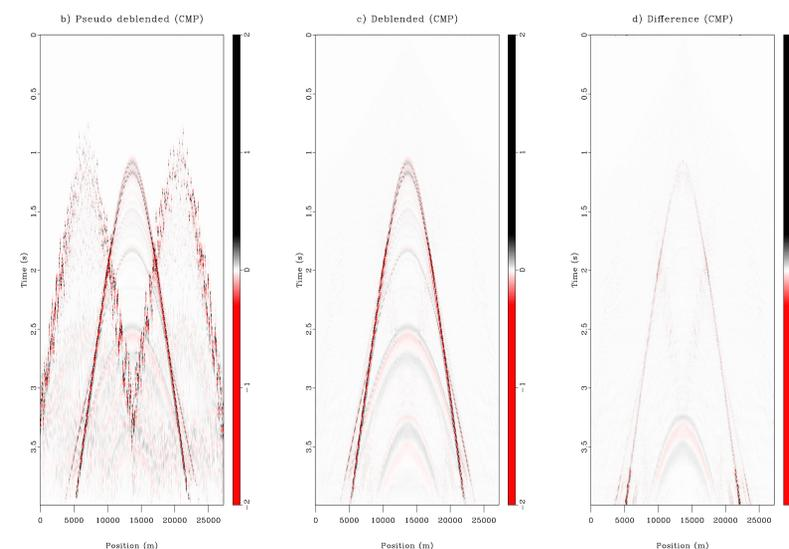
Figure 4: Wedge model results in CMP: Deblending of a two simultaneous source survey in CMP domain with a) unblended data, b) pseudo-deblended data, c) deblended data, and d) difference respectively.
