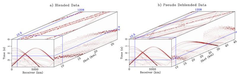
Figure 1: Blended vs pseudo deblended data: Blended data in a) and pseudo deblended data in b), it can be seen that the shots that belong to each coordinate set show up as coherent in other domains while shot interference shows up as dithered.
