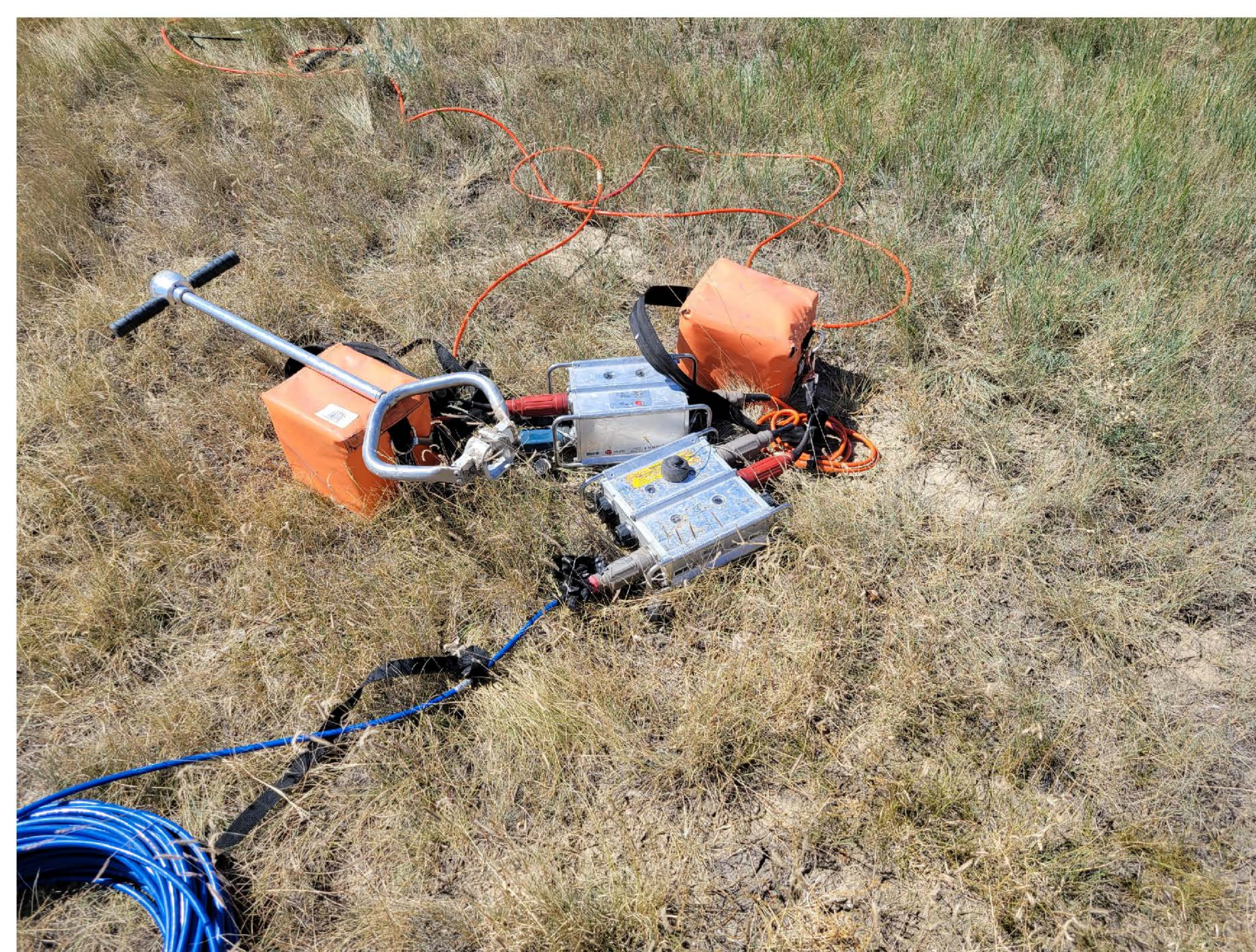
Aries 3C Ram (top silver box) and line tap used for collecting reflection seismic.
