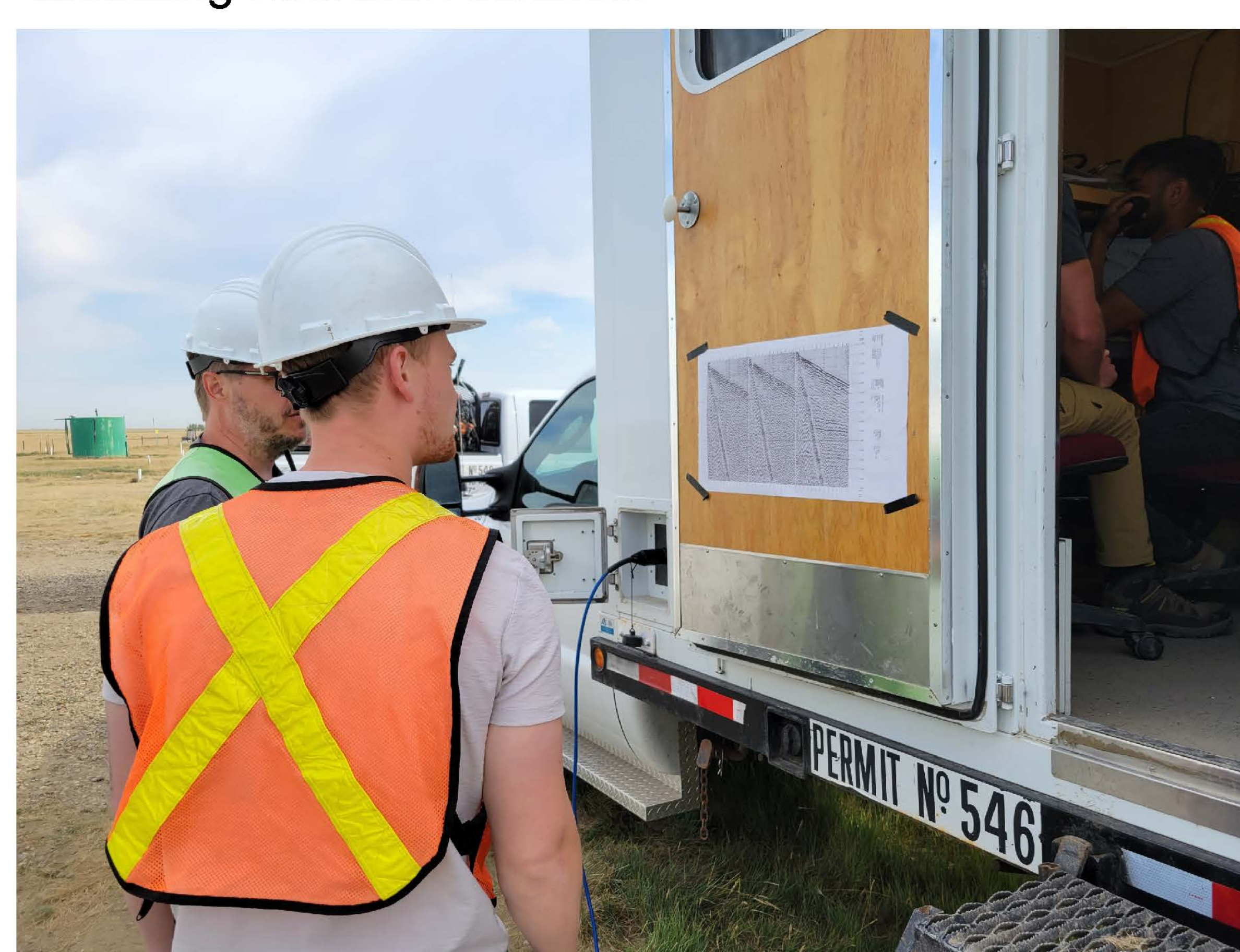
A student discussing the results of a single source point reflection record. First breaks, air blast, and a reflection can be seen in the rightmost section on the record taped to the door.
