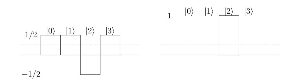
▶ Reading stage reads the correct model,  $|2\rangle$ , with probability 1. Bigger problems need more iterations.
