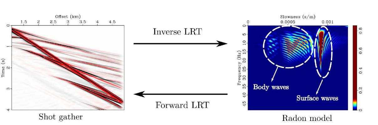
Linear Radon Transform: a The inverse LRT is used to estimate the Radon model (right) from the shot gather (left). The Radon model allows to identify the zones of body and surface waves in the frequency-slowness domain. The seismic shot gather is reconstructed by applying the forward LRT.
