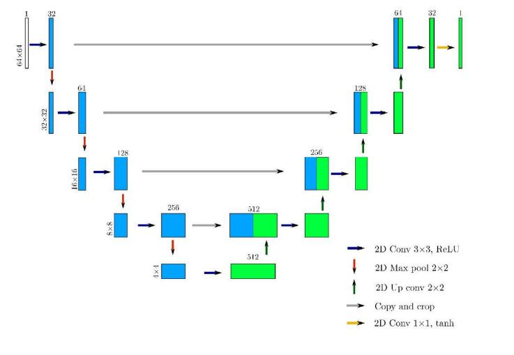
**Unet**: We use the Unet to predict the Radon model of seismic shot gathers without surface wave noise.
