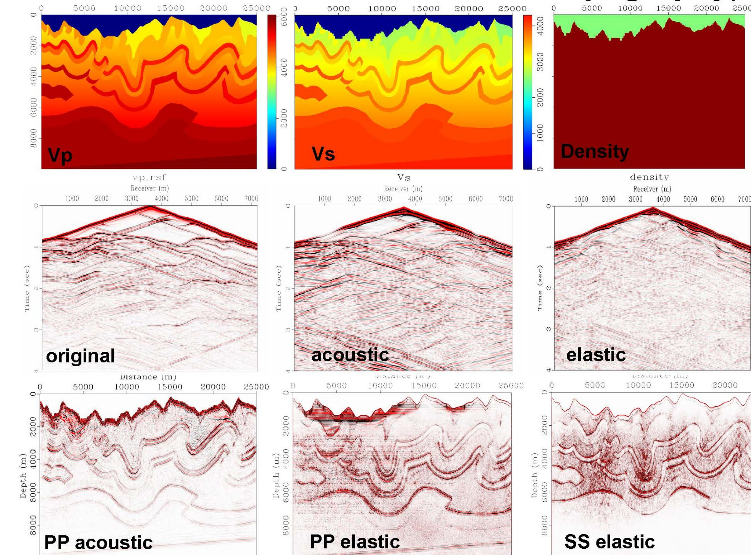
In the Figure above, we see a comparison between acoustic and elastic modelling and RTM, in all cases from topography. The elastic migration includes near surface noise, but the acoustic does not.
