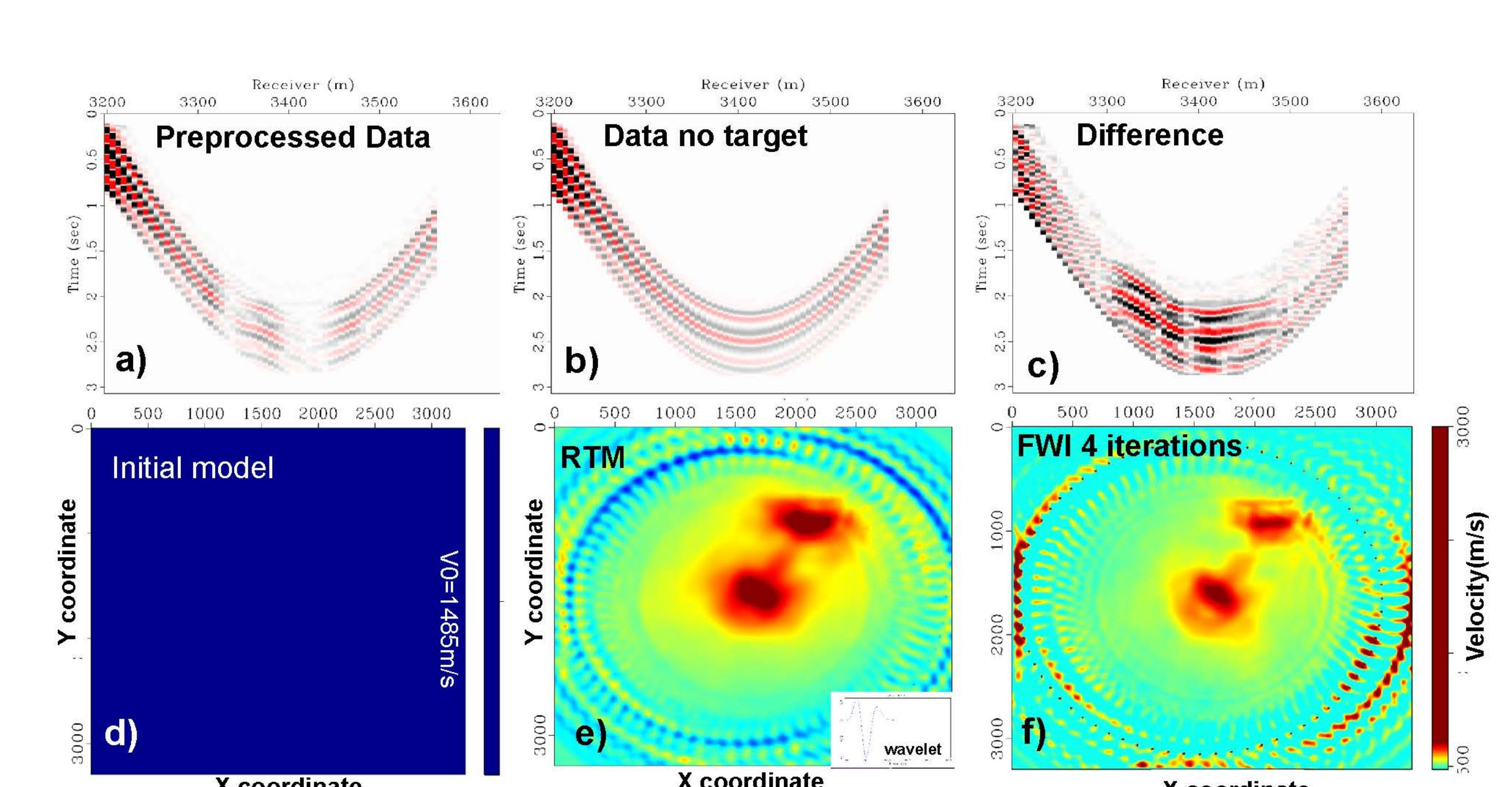
All real physical model: a) Original shot after mute, b) Original shot without target. c) Difference, d) Initial model, e) RTM from difference, f) real data FWI (from difference)
