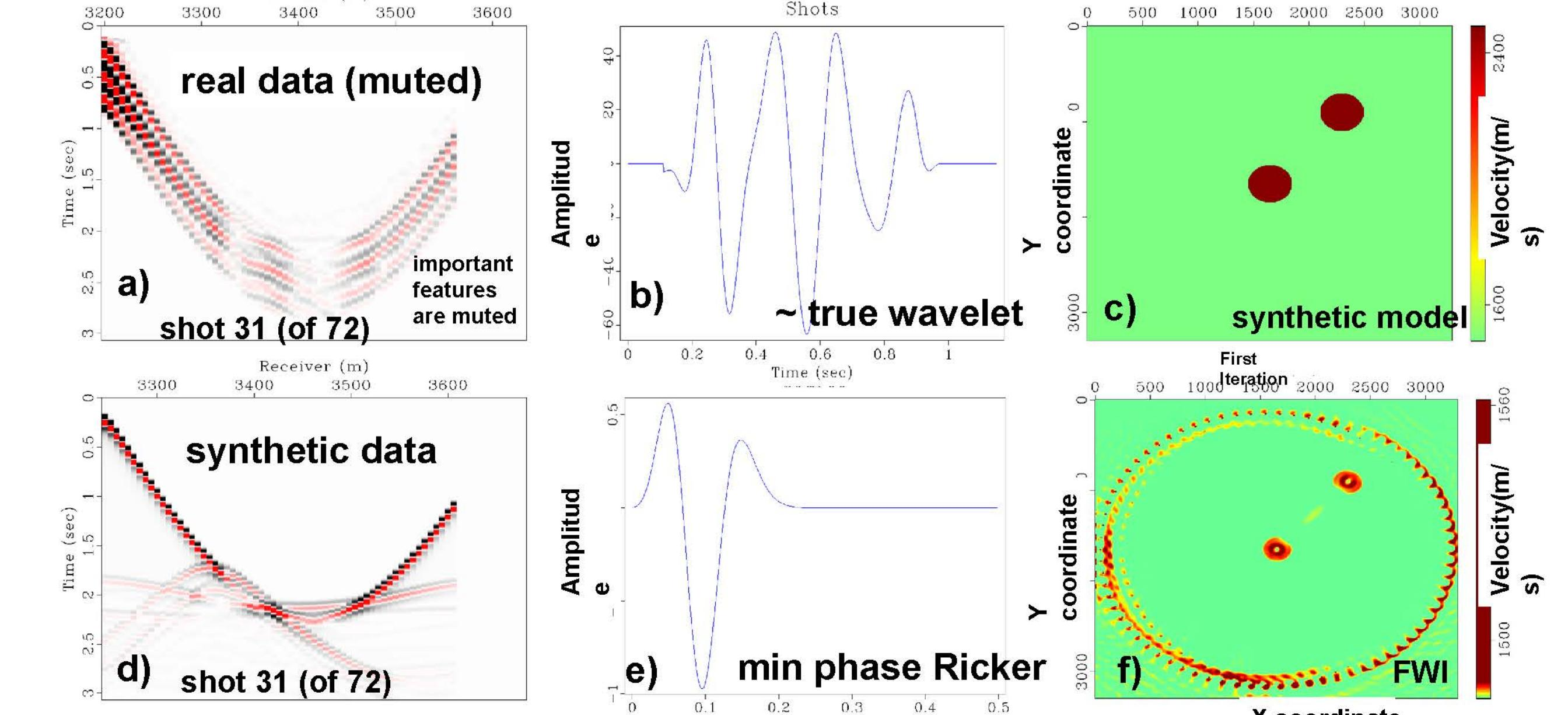
In this example, we work first with matching synthetic data to understand the problem a) Original shot from physical model after mute, b) true wavelet. c) fake velocity model, d) shot from fake numerical model e) Ricker wavelet, f) FWI from synthetic (inverse crime).
