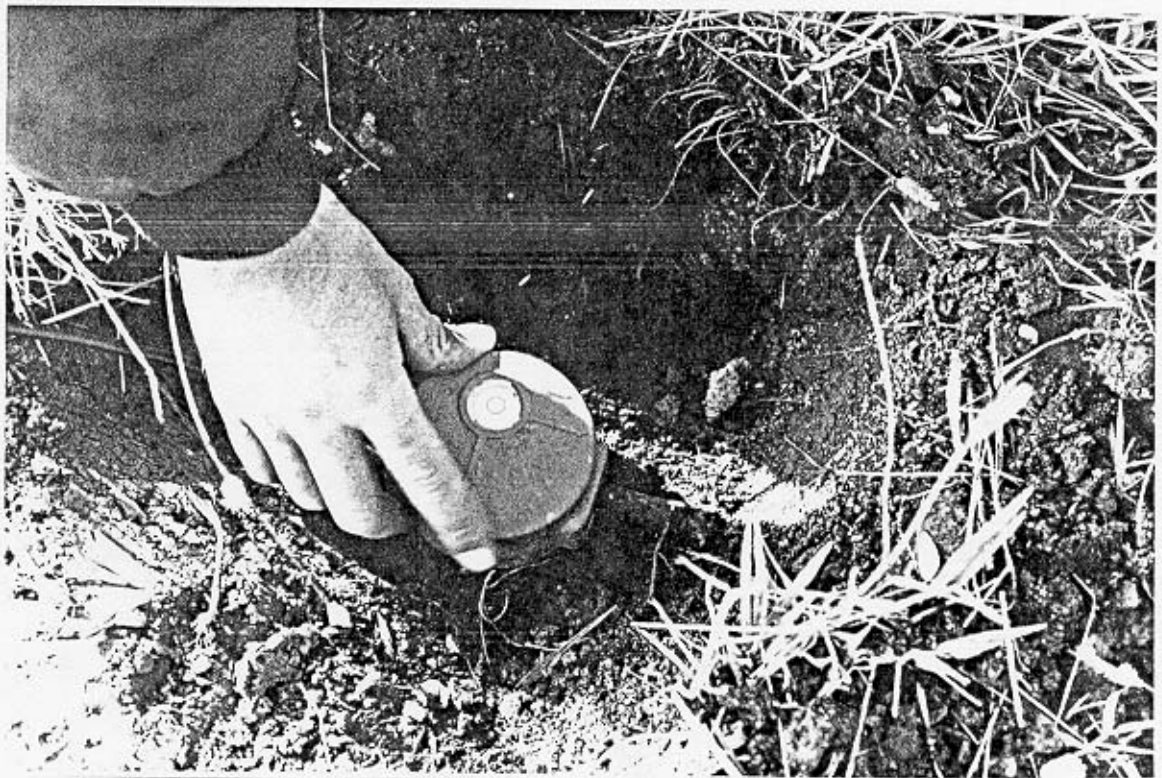
FIG. 2. A 3-component OYO geophone in position, showing the leveling bubble and orientation arrows.
