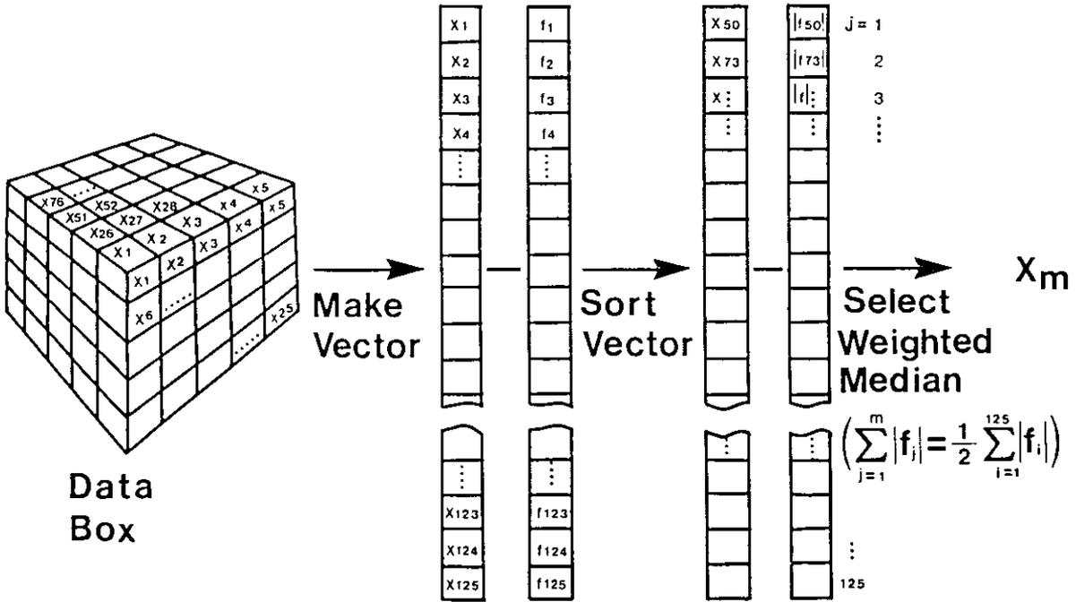
FIG. 4. (c) Schematic diagram of the 3-D median filter process with filter coefficients.
