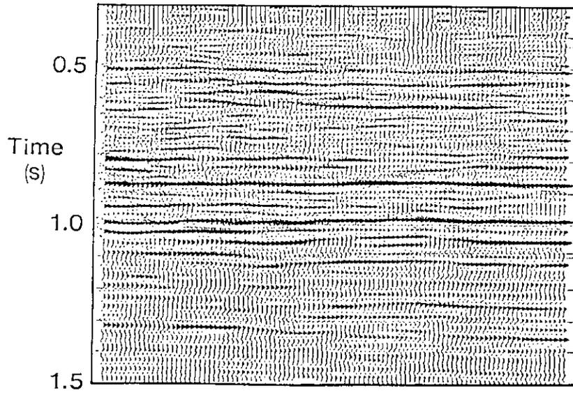
FIG. 6. (b) Same line extracted from the 3-D volume after mean 3-D f-k filtering,
