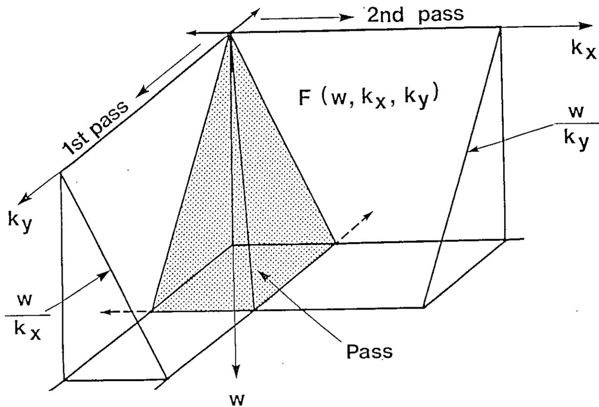
FIG. 2. (a) Schematic diagram in f-k space of a two-pass 2-D filter,
