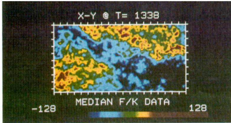
FIG. 7. (c) The same time slice after median F-k filtering.
