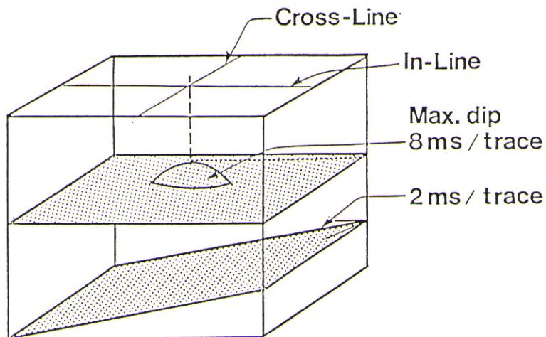
FIG. 3. (a) 3-D model geometry with a hemispherical anomaly,
