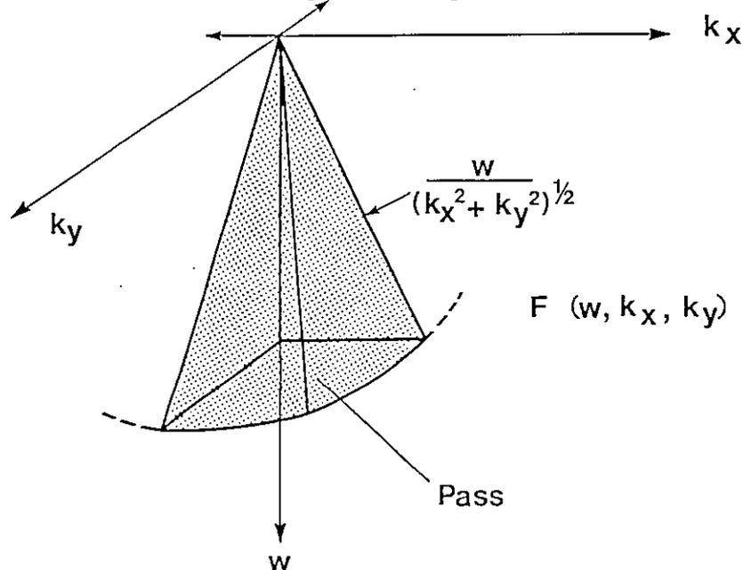
FIG. 2. (b) Schematic diagram in f-k space of a one-pass 3-D f-k filter.
