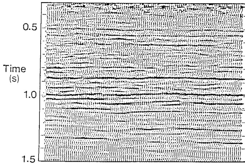
FIG. 6. (c) Same line extracted from the 3-D volume after median 3-D f-k filtering.
