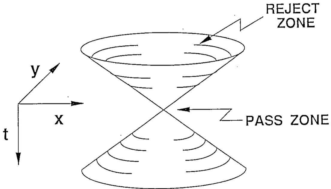
FIG. 1. Conical pass and reject regions of a 3-D filter.
