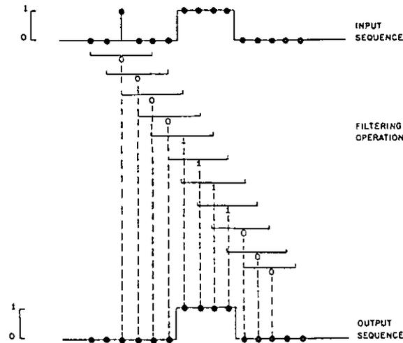
FIG. 4. (a) Schematic diagram of the 1-D median filtering process with a 5-point window,
