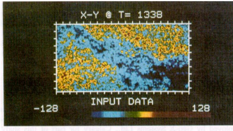
FIG. 7. (a) Time slice of 3-D data volume at 1.338s through the top of the faulted carbonate of interest,
