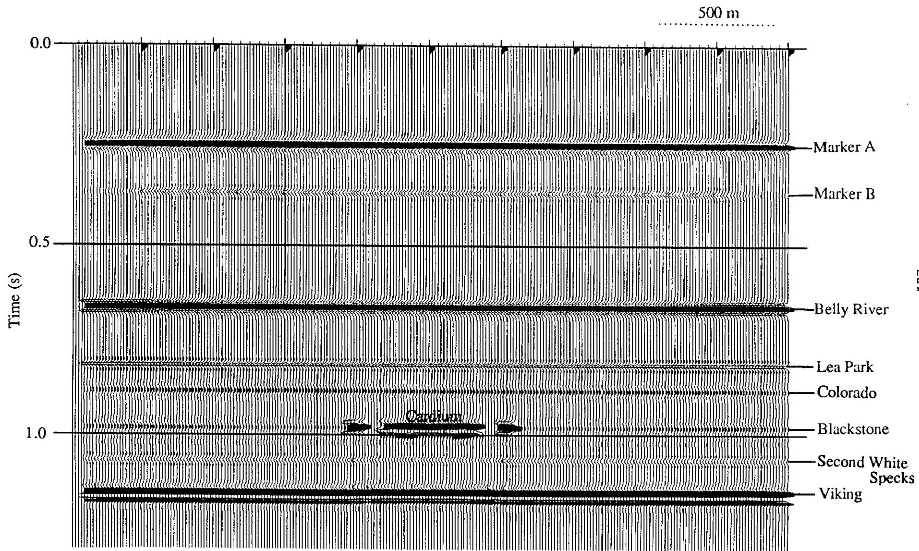
Figure 14: Final P-P synthetic stack section
