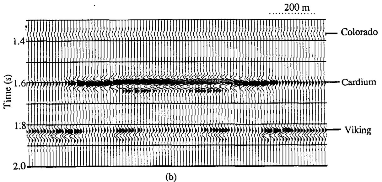
Figure 13: Comparison between (a) the surface seismic P-Sv anomaly and (b) the modeled P-Sv anomaly
