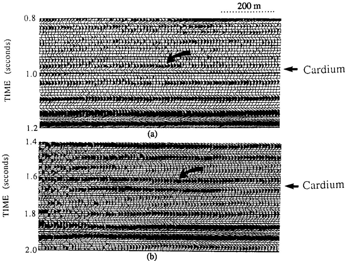
Figure 2: Carrot Creek Cardium amplitude anomalies on (a) the vertical and (b) the radial component of CCSW01
