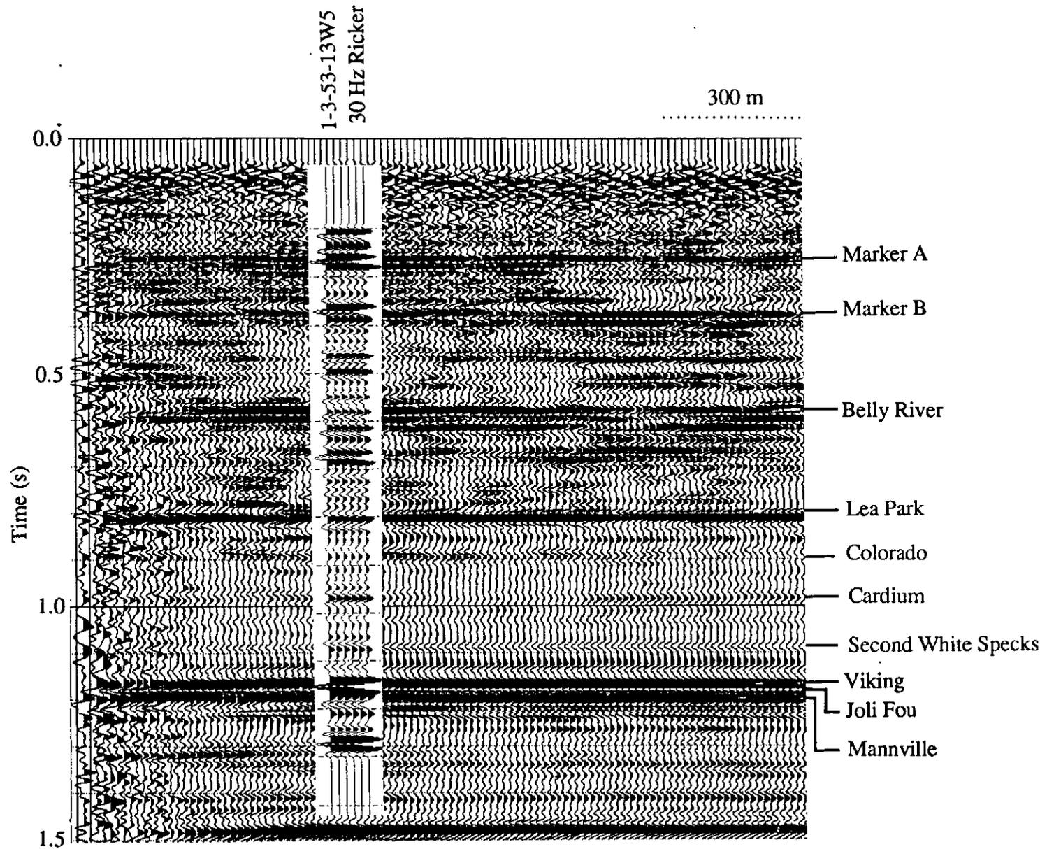
Figure 6: Correlation of a P-wave synthetic with the vertical component of line CCSW01
