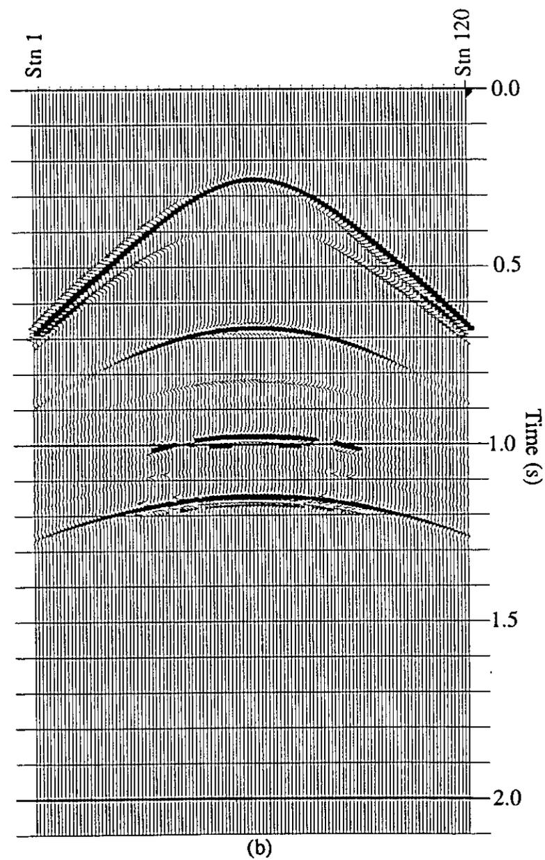
Figure 9: Radial (a) and vertical (b) component synthetic shot records (shot 15) from the Carrot Creek Model
