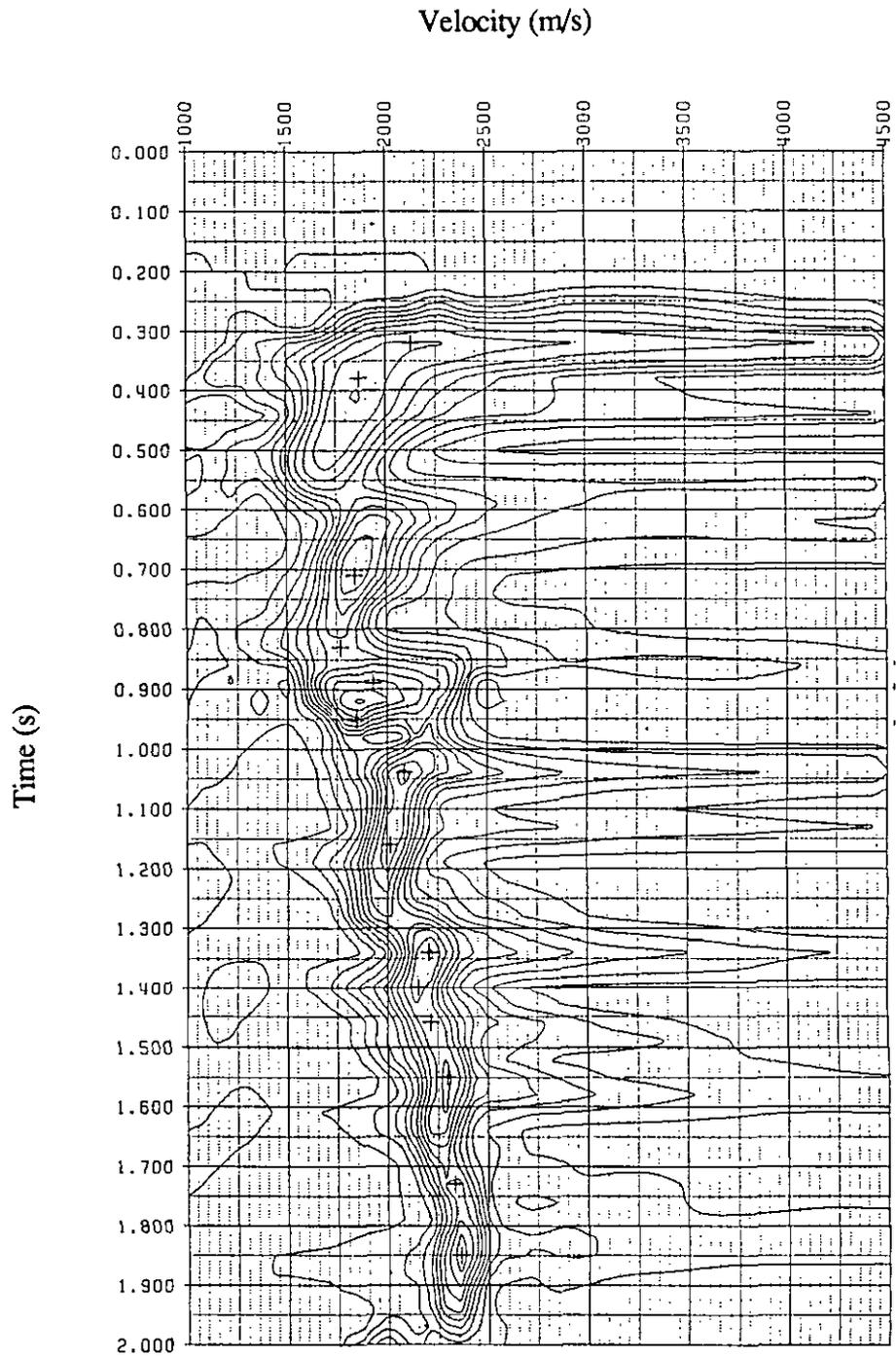
Figure 11: Velocity analysis of the P-Sv synthetic data
