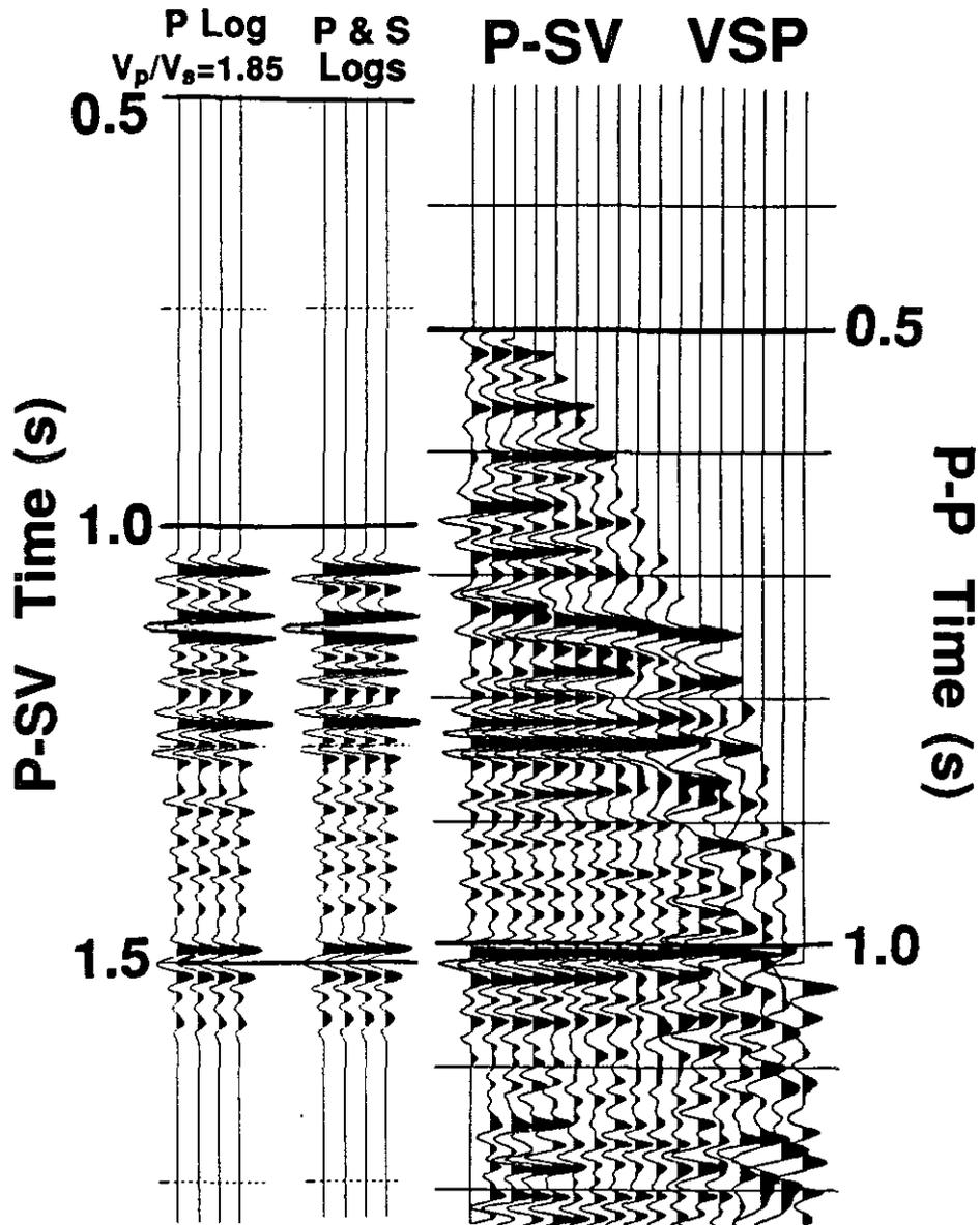
FIG. 5. The P-SV map from Rolling Hills compared to the P-SV synthetic stack created using a full waveform log (center), are a P-SV synthetic stack (left) created using the P-wave log only and an assumed  $V_p/V_s=2$ .
