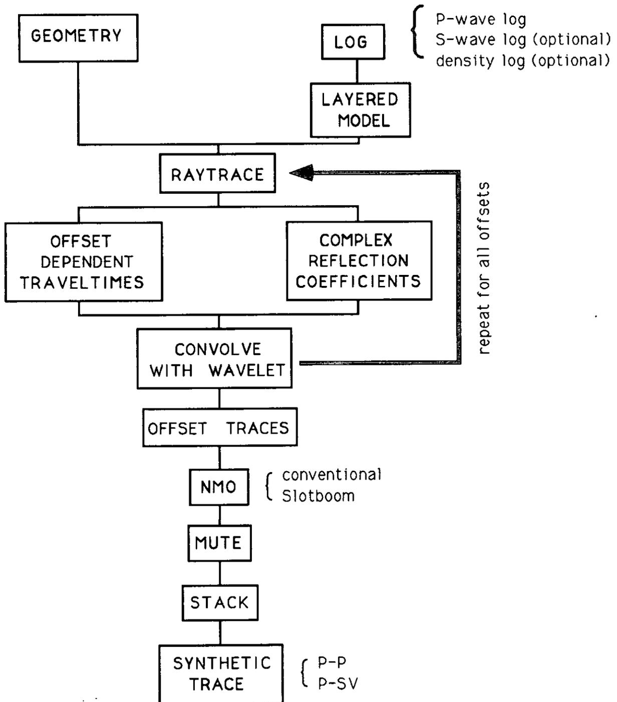
FIG. 2. Flowchart of the general steps followed to produce synthetic stacks.
