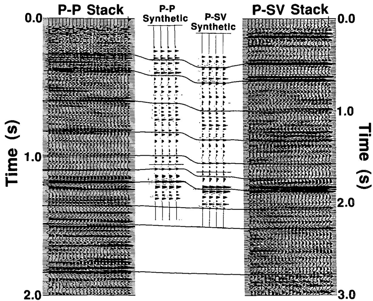
FIG. 7. Carrot Creek P-P section compared with P-P synthetic stack and P-SV section compared with P-SV synthetic stack (Nazar and Lawton, 1991).
