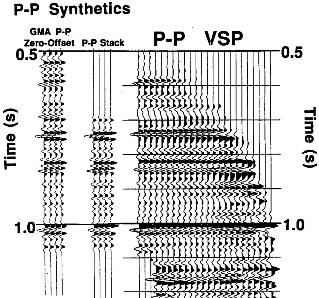
FIG. 4. GMA zero offset P-P synthetic seismogram and the P-P synthetic stack for five offset from 300 m to 500 m, compared with the P-wave map from the Rolling Hills VSP.
