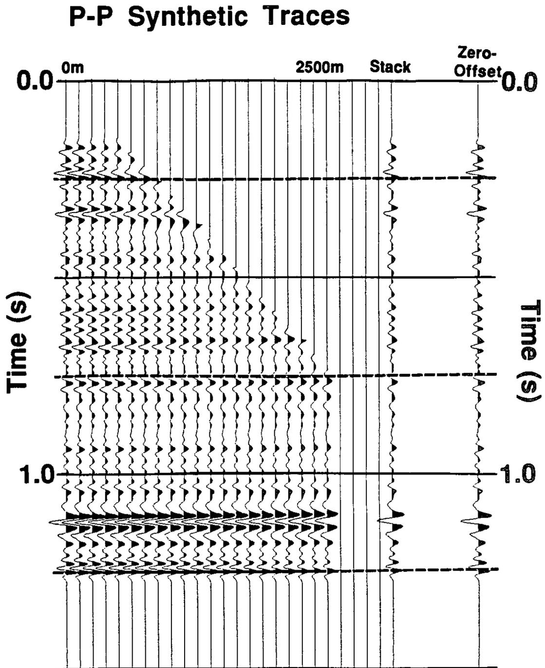
FIG. 8. P-P synthetic gather for offsets of zero to 2500 m and a comparison of P-P synthetic stack with the P-P zero-offset synthetic.
