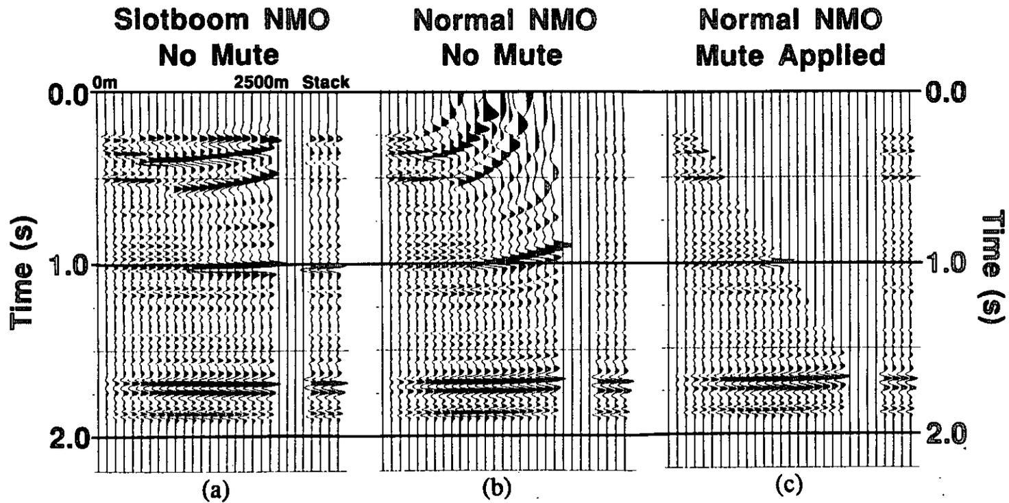
FIG. 6. P-SV synthetic gathers for offsets of zero to 2500 m. (a) with Slotboom NMO applied. (b) with normal NMO applied. (c) with normal NMO and mute applied.
