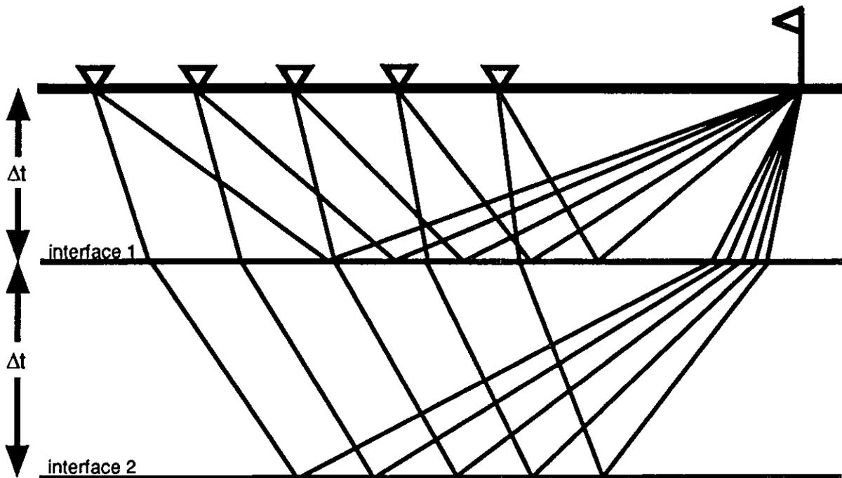
Figure 3. Model of constant traveltimes layers raytraced at multiple offsets to produce traces for stacking into a P-SV synthetic stack.
