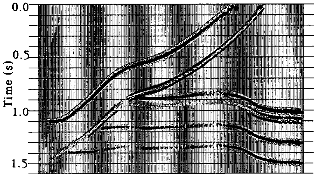
FIG. 5. Result using depth-variant common conversion point (CCP) binning for Highwood Structure PSV synthetic seismic section.
