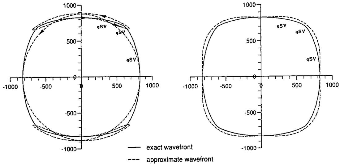
FIG. 5: Exact and approximate wave surface of Dog Creek shale. The approximation is carried out
