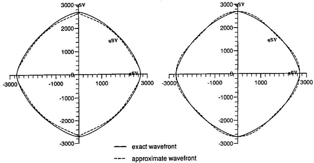
FIG. 3: Exact and approximate wave surface of Mesaverde mudshale. Notice the large near-vertical decrease of the exact ray velocity, though the extreme near-vertical change of the exact curvature can hardly be seen. The approximation is carried out
