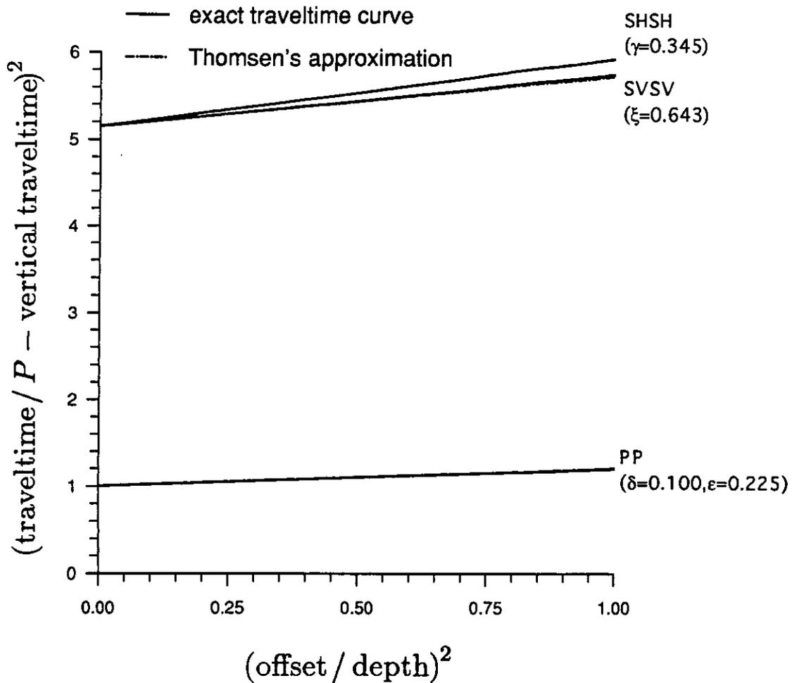
FIG. 6: Exact and approximate traveltime curves of Dog Creek shale. Due to no convexity of the SVSV traveltime curve indicated by a large positive anisotropy coefficient  $\xi$ , Thomsen's (1986) approximation of the NMO velocity is excellent in spite of a less perfect approximation of the wavefront.
