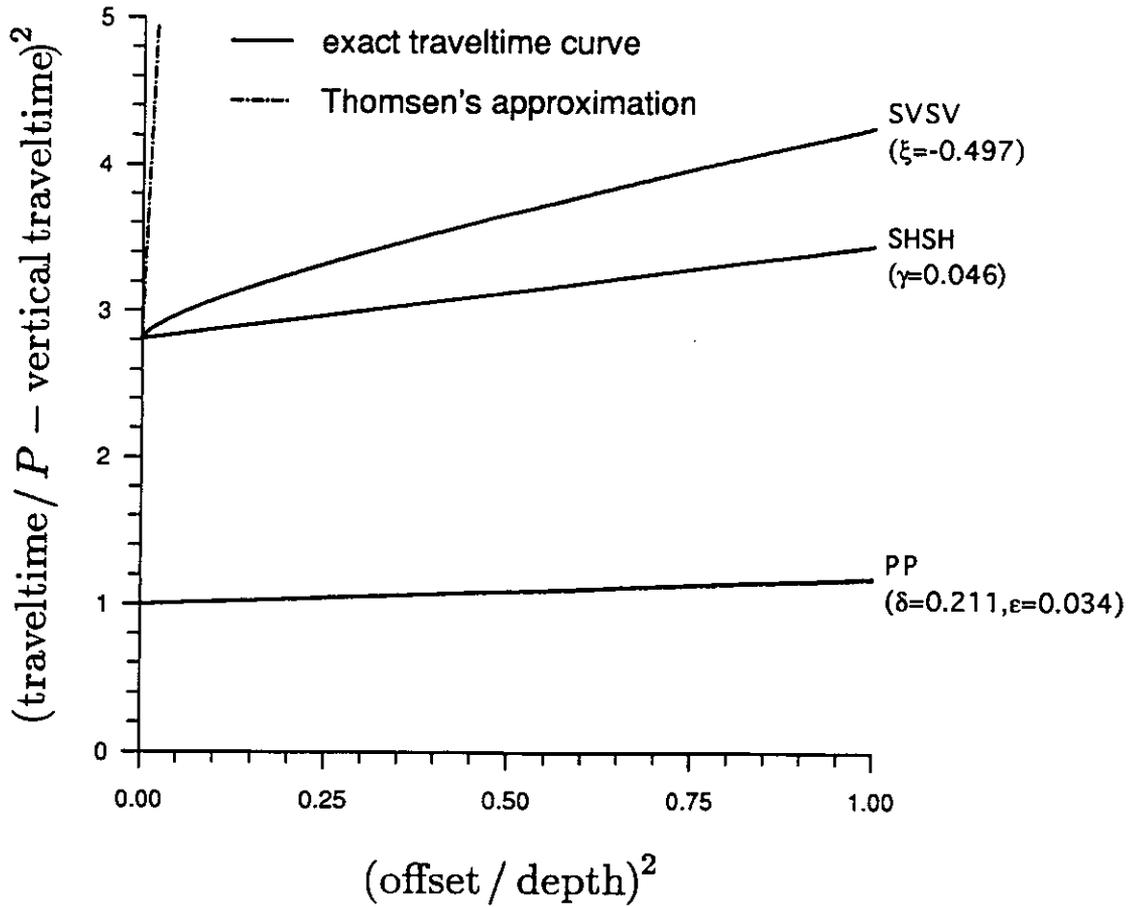
FIG. 4: Exact and approximate traveltime curves of Mesaverde mudshale. Due to the strong convexity of the SVSV traveltime curve indicated by a large negative anisotropy coefficient  $\xi$ , Thomsen's (1986) approximation is valid only in the immediate neighbourhood of near-vertical incidence. In contrast, the PP traveltime curve is hardly influenced.
