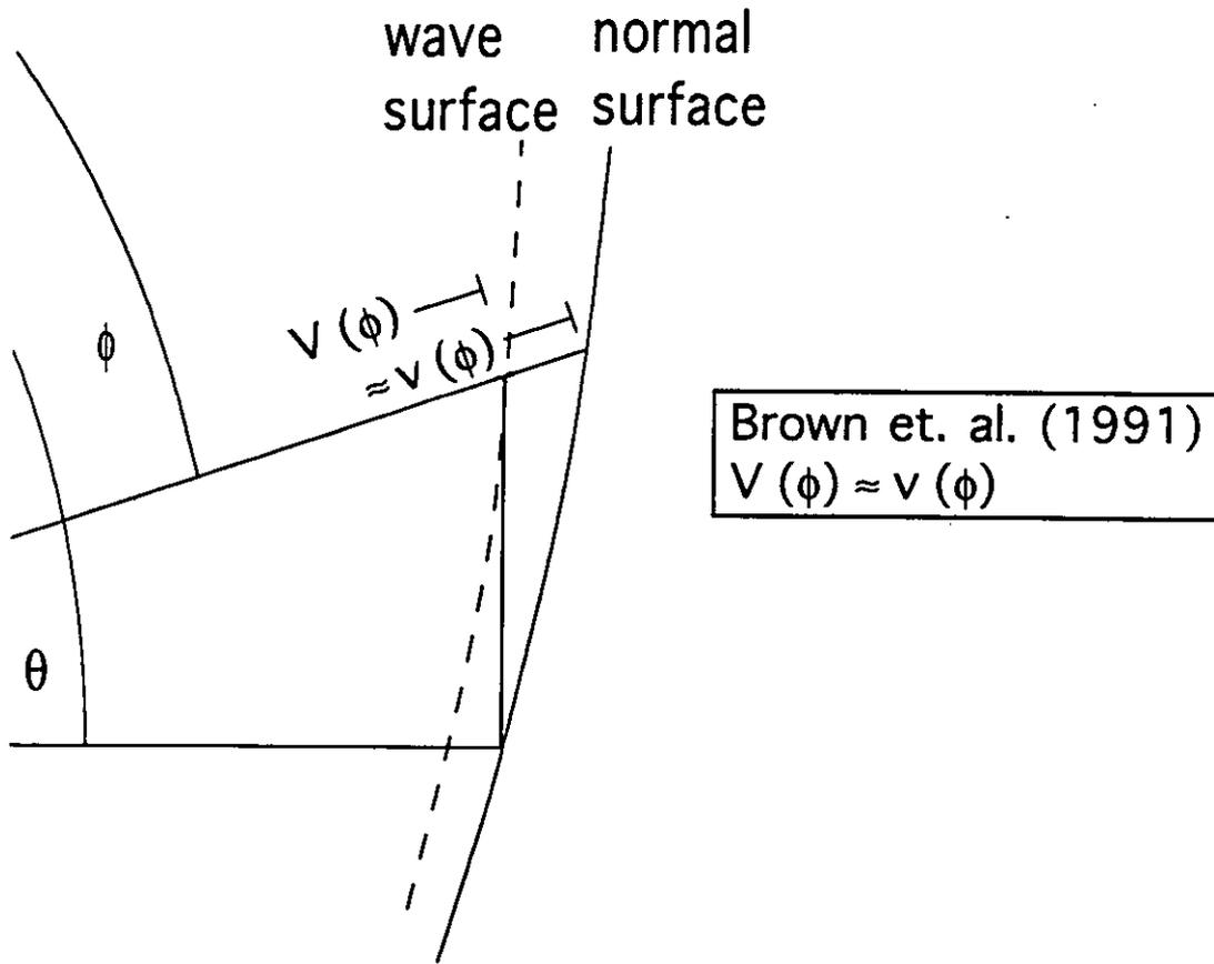
FIG. 1b: Different approximations of the exact ray velocity. Physically, a phase angle  $\theta$  is assumed to correspond to a ray angle  $\phi$ . Here, an approximation of Brown et al. (1991) is illustrated. The enlargement shows parts of the normal and the wave surface as well as (from the bottom to the top)
