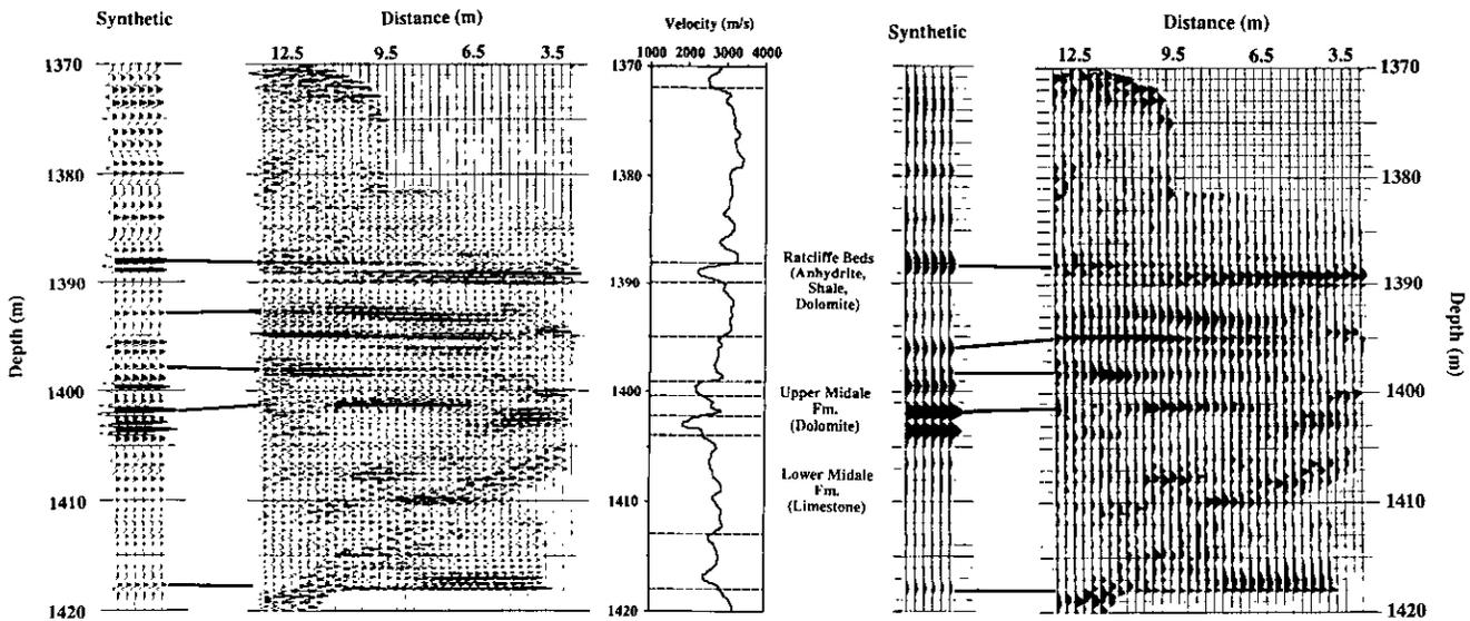
Figure 16. Display of final interpretations of cross-well reflection S-wave data. Downhole sources commonly generated considerable S-wave energy. a.) S-wave synthetic seismogram generated from S-wave sonic log shown in c.). b.) Final cross-well section from stack of nine receiver maps. c.) S-wave sonic log. d.) Instantaneous amplitude of synthetic seismogram in a.) e. The instantaneous amplitude of the final section in b.) (After Khalil *et al.*, 1993.)
