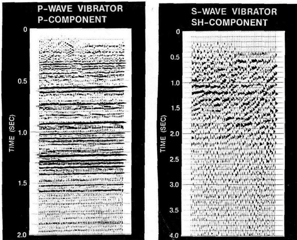
Figure 5. Examples of P and SH wave stacked data (Brute Stack) from the early Conoco Vibroseis project. Improved processing and vibrator controls have greatly improved the overall data quality in recent years.
