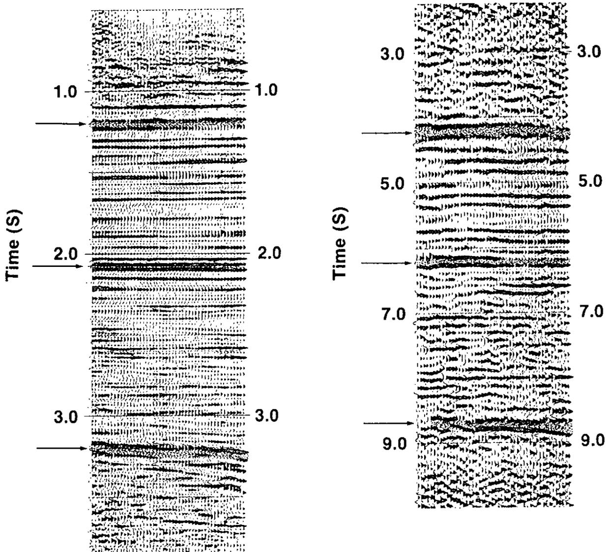
Figure 13. P- and SH-wave expanded reflection sections gather in southern Louisiana. The arrow marks show the correlation in the reflection events between the P- and S-wave data, as well as the VSP data in Figure 14. (After Corbin *et al.*, 1987)
