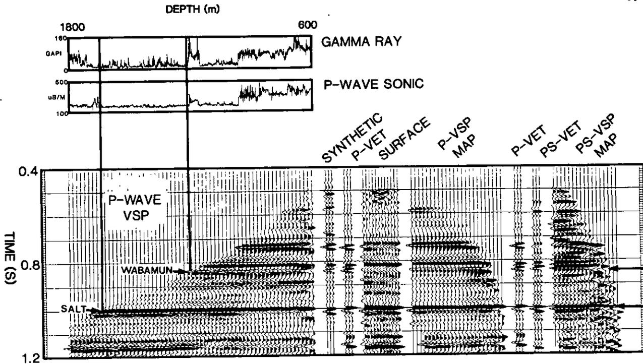
Figure 15. Display incorporating various P-wave and P-SV wave data. In particular, P-wave VSP reflection data is at left hand side of the display, and P-SV reflection data at the far right hand side of the display. Event are correlated, and all time traces are displayed trace normalized. (After Geis *et al.*, 1990.)
