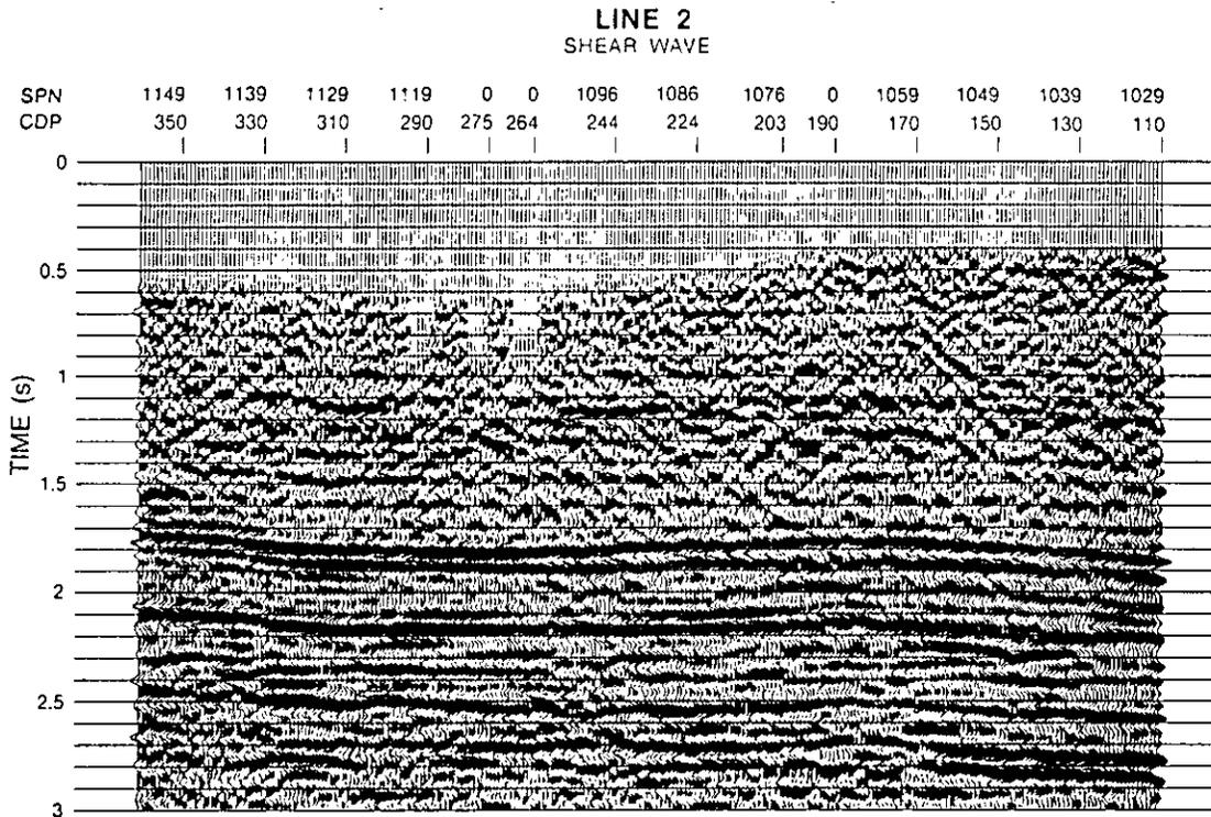
Figure 9. Stacked CMP P- and SH-wave sections for line 2 of the Empire-Abo field. The Morrow sand is near a reflection time of 1.25 s on the P-wave data and 2.5 s on the S-wave data. (After McCormack *et al.* 1985.)
