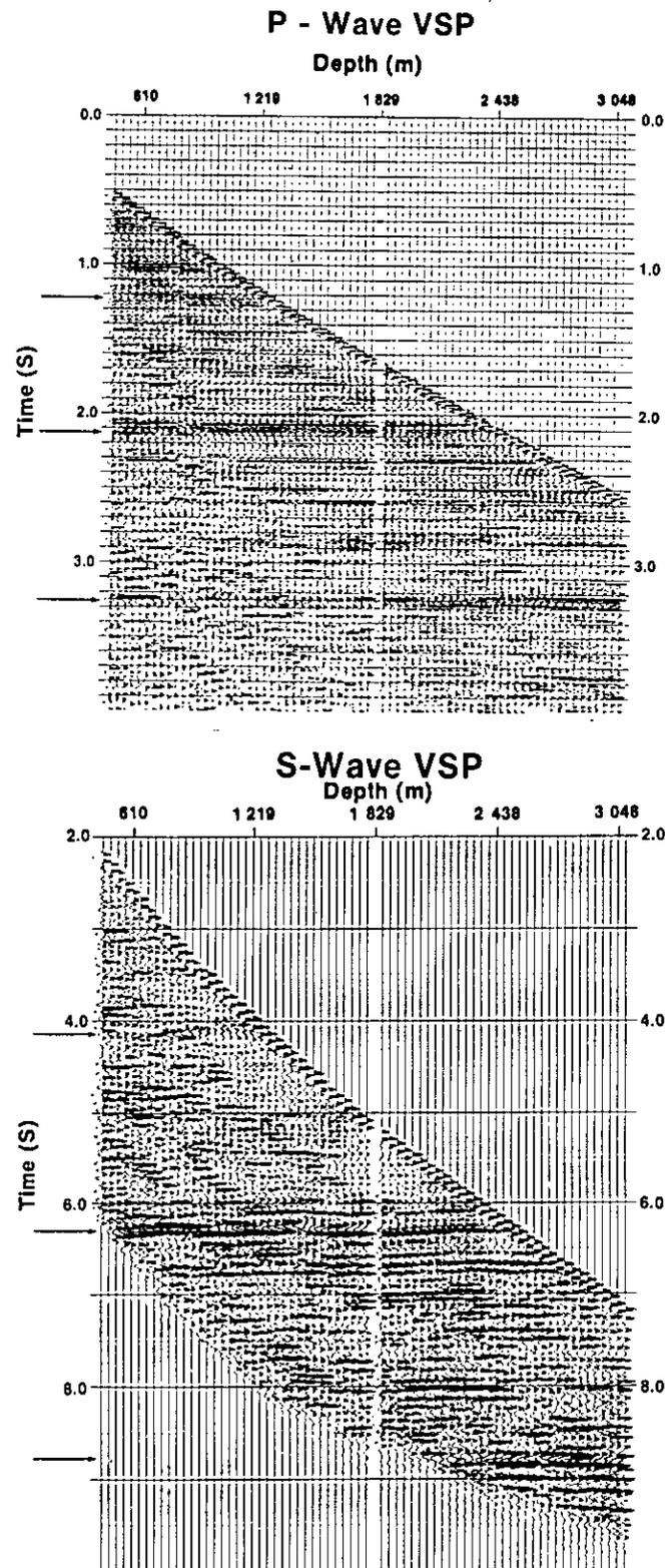
Figure 14. Upgoing P- and S-wave reflection events from VSP data gathered at the same location as the expanded reflection line of Figure 13. Flat-lying events are primary reflections. The three arrows mark reflections which are correlated to the surface reflections of Figure 13. (After Corbin *et al.*, 1987.)
