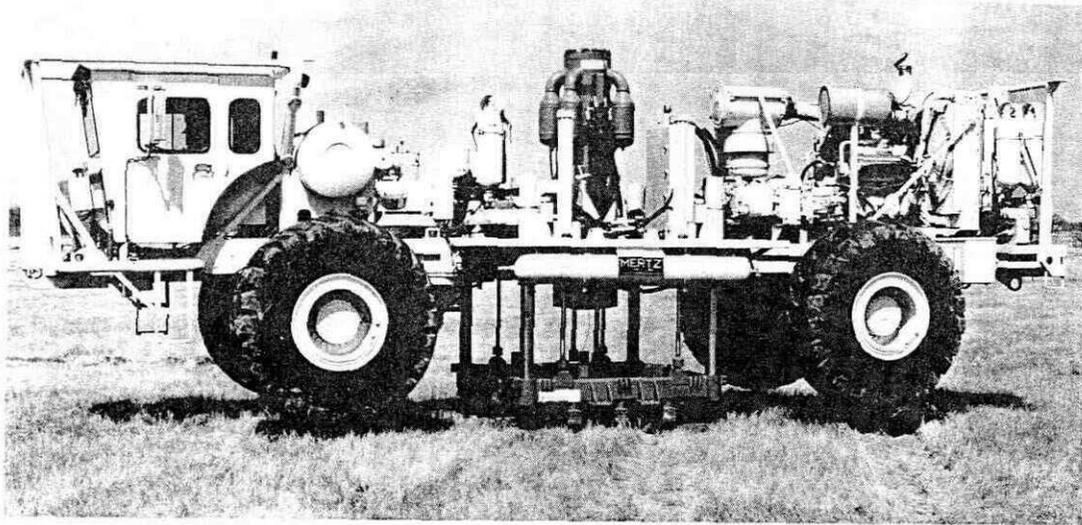
Figure 4. ARIS impactor seismic source. The polarized impulsive surface source is capable of generating directed impulses which can be resolved into three orthogonal source polarizations (P, SV, and SH) without changing the vehicle orientation.
