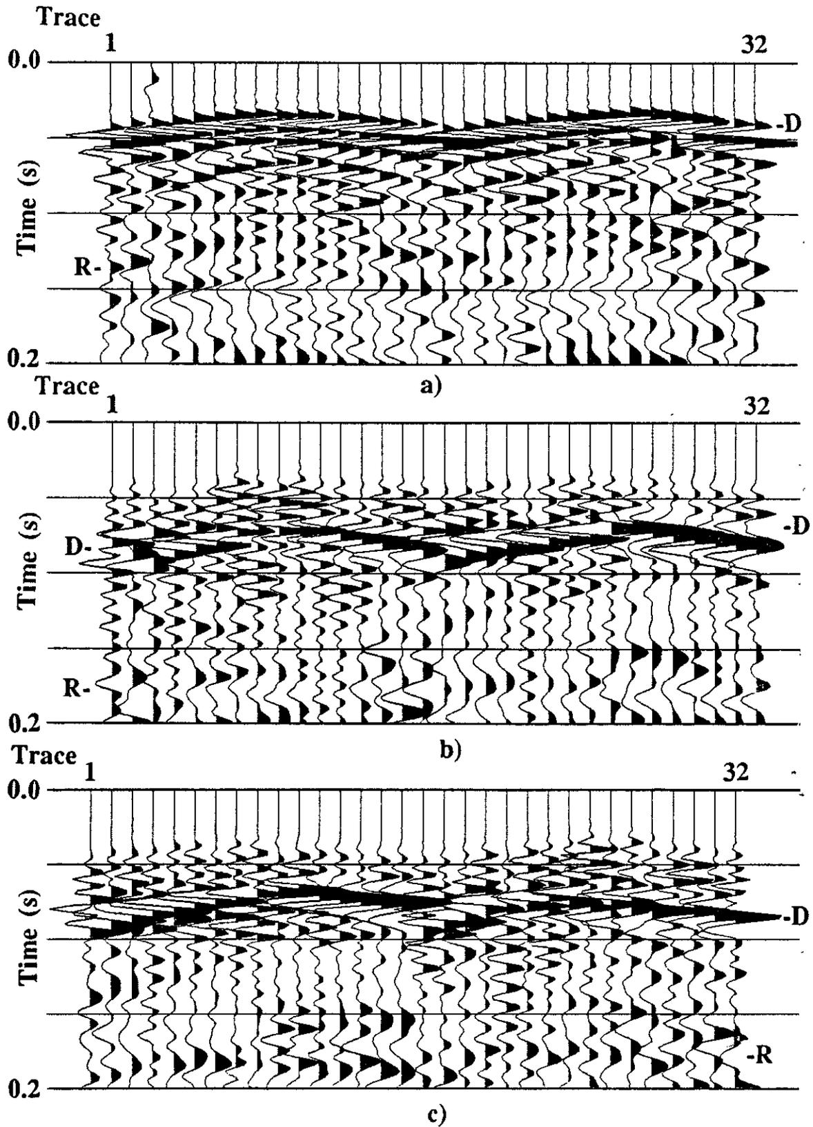
FIG. 3. Shot gathers for a) vertical, b) east-west, and c) north-south oriented components. Shot at 16 m depth. Traces 17-32 of b) and 1-16 of c) are radial. Direct arrivals - D.
