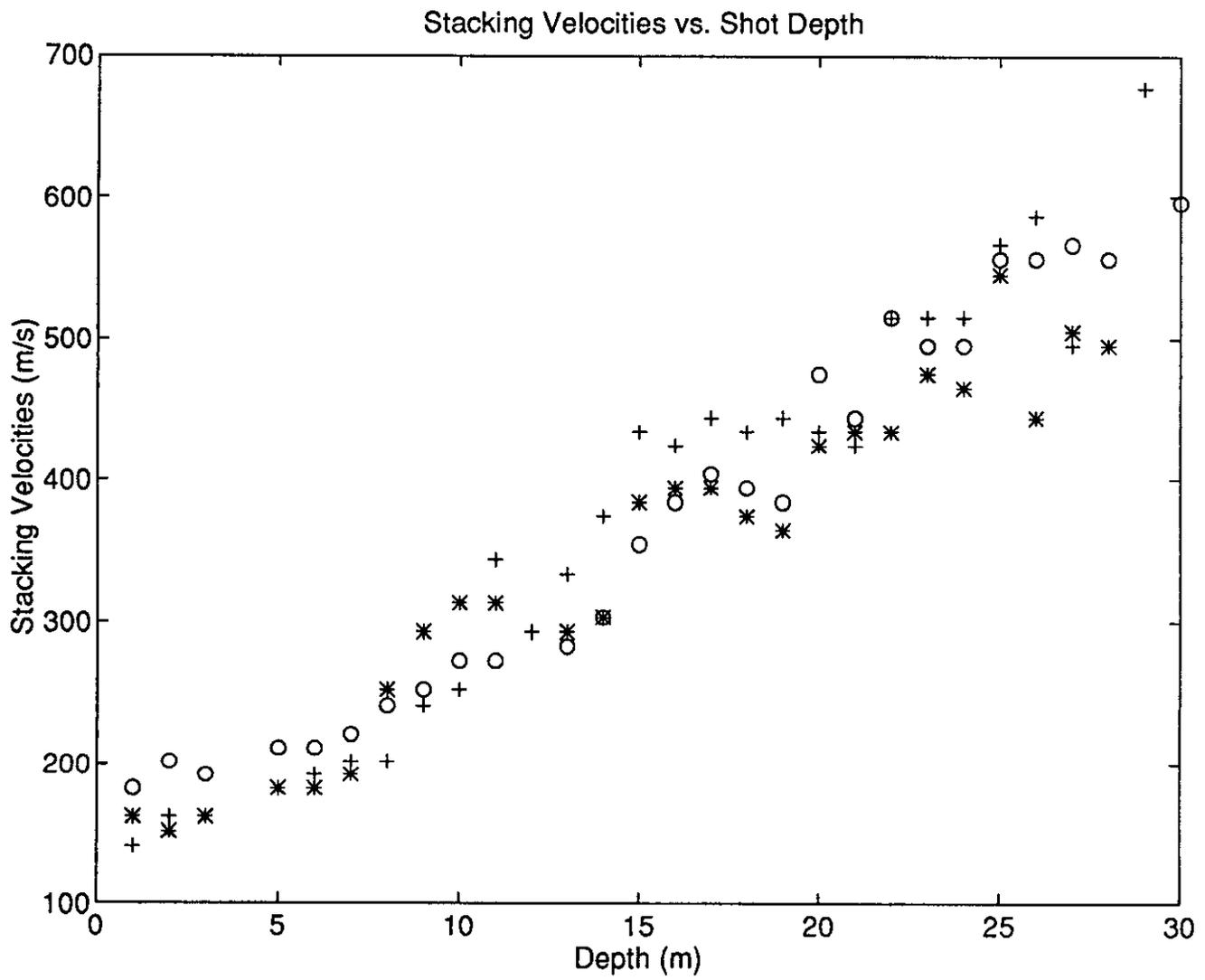
FIG. 10. Stacking velocities for radial records. NMO in the direct arrivals will be compensated for by these velocities (o = vertical component, + = east-west component, \* = north-south component).
