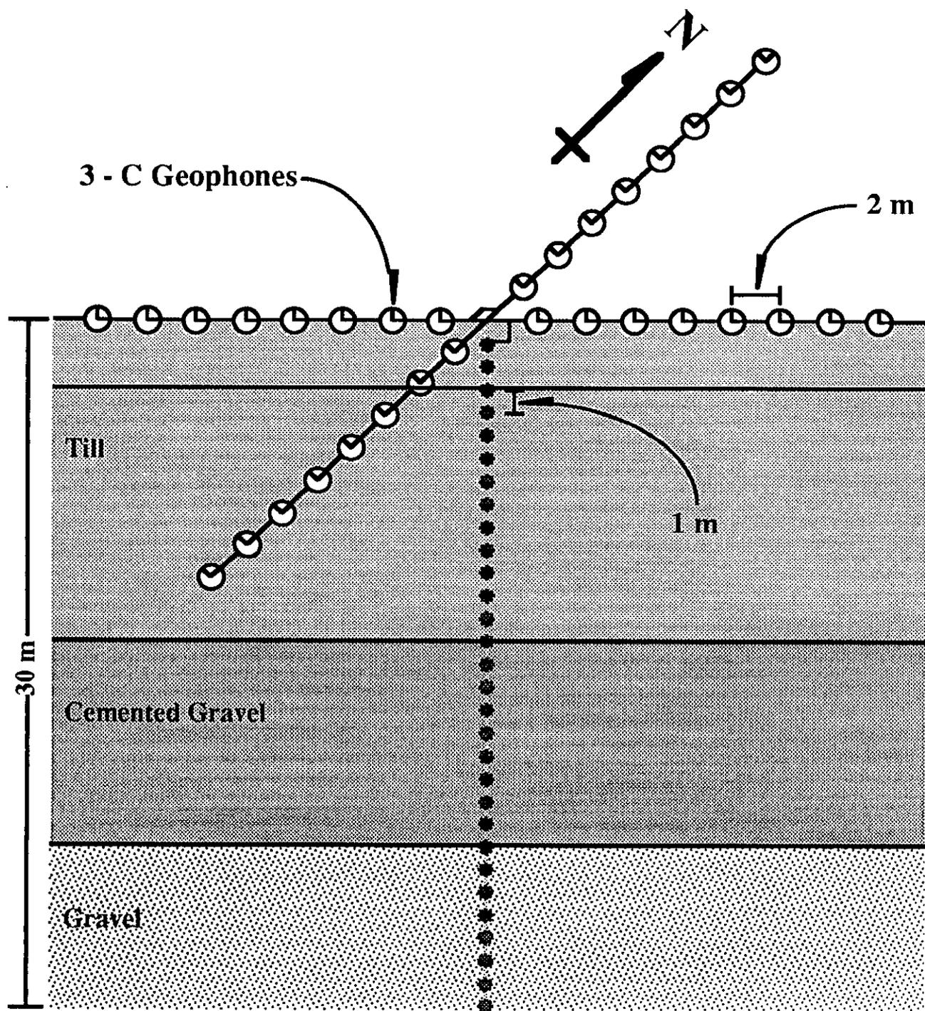
FIG. 1. Survey geometry and geological interpretation.
