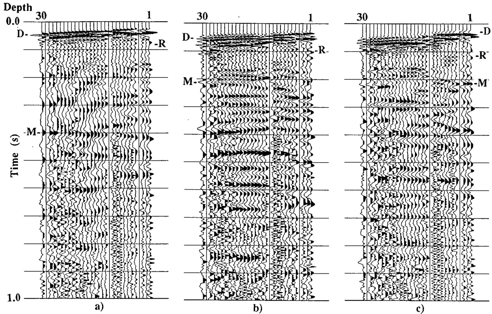
FIG. 11. Common receiver gathers for receiver 10 (4 m south of borehole). a) vertical, b) radial, and c) transverse. Direct arrivals (D), Reflections (R), Multiples (M). 125 ms agc applied. Bandpass filtered at 5/10-120/180 Hz.
