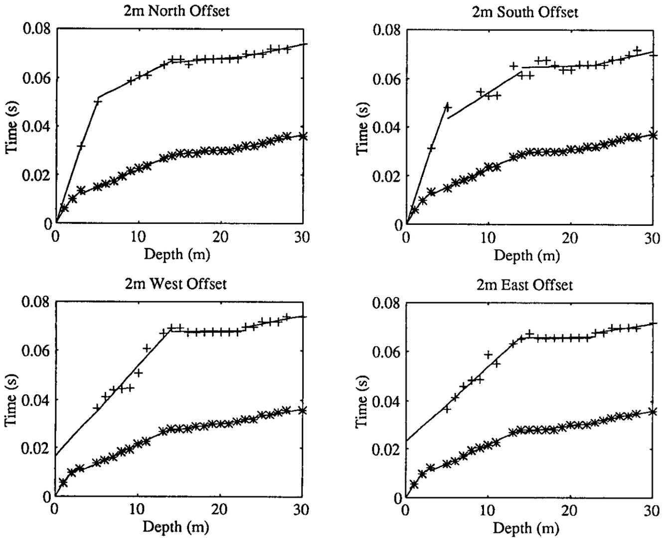
FIG. 5. Time/depth curves for the near offset (2m) receivers (+ = radial component, \* = vertical component).
