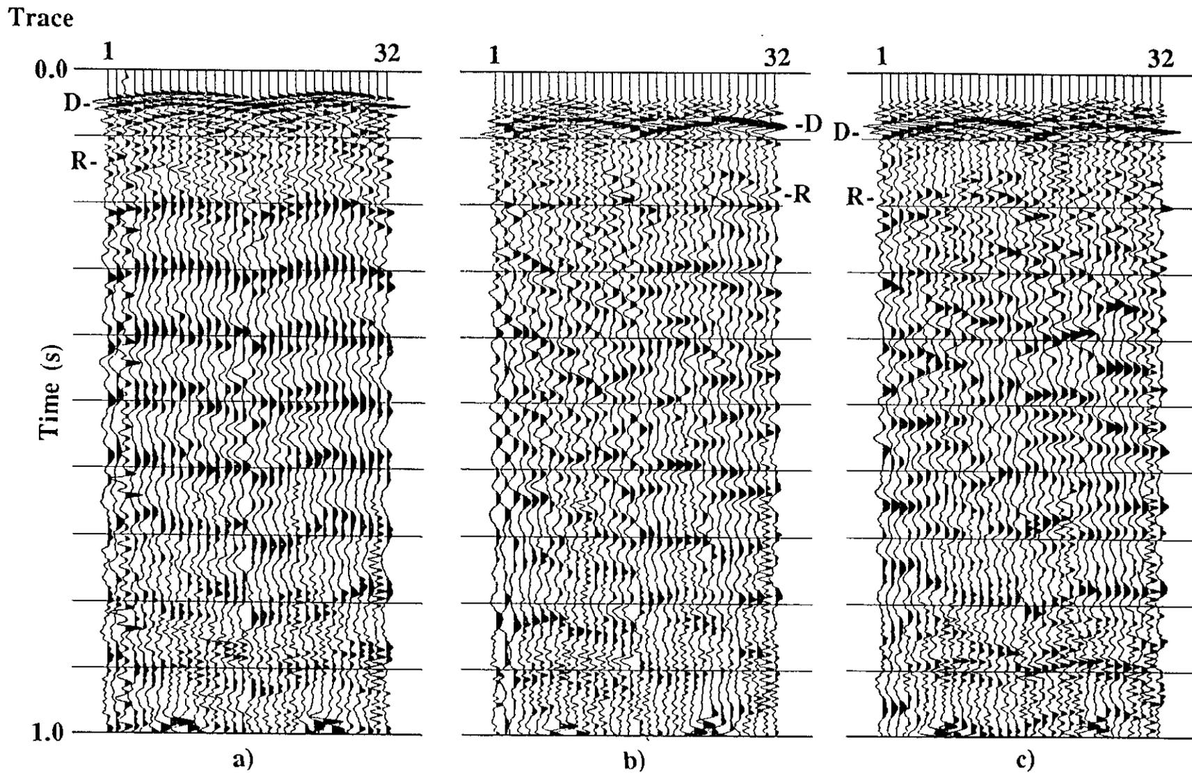
FIG. 2. Shot gathers for a) vertical, b) east-west, and c) north-south oriented components. Shot at 16 m depth. Traces 17-32 of b) and 1-16 of c) are radial. Direct arrivals - D, Reflections - R.
