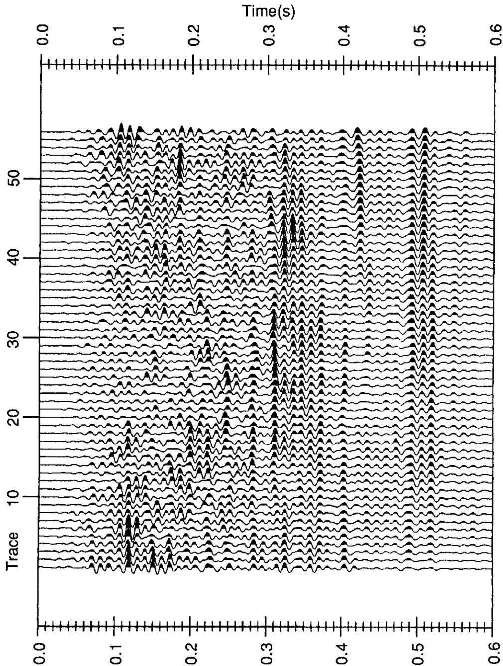
FIG. 7. Same line as in Figure 6 but from the reprocessed 1990 data set. The Devonian reflector is at about 0.5 s. There is a time shift between the original and the reprocessed data even though they are supposed to have the same datum of 600m. The event at 0.31 s, just above the Grand Rapids Formation, is stronger and more continuous than in Figure 6.
