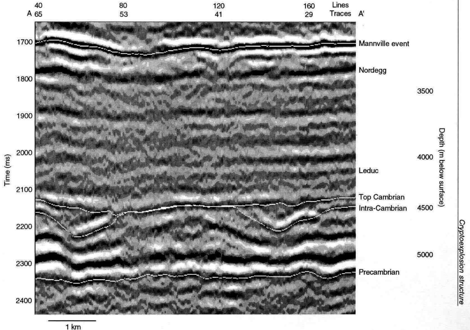
FIG. 5. NW-SW seismic line over the cryptoexplosion structure with interpreted horizons. The truncation of dipping events beneath the Top Cambrian unconformity and the eroded central uplift are seen clearly.
