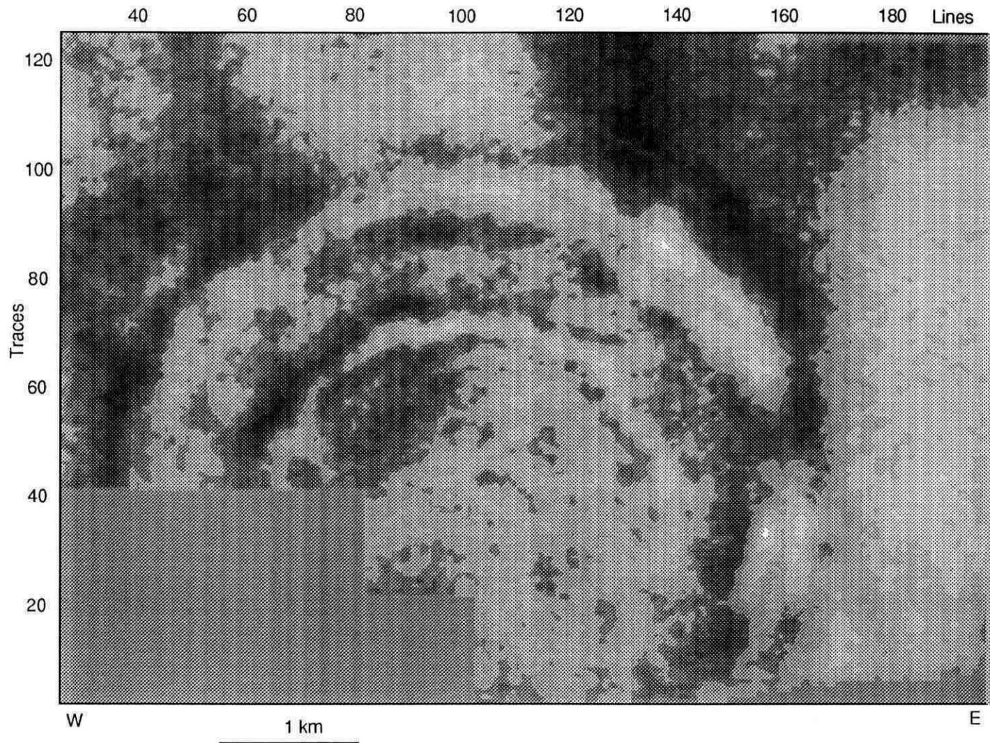
FIG. 7. Horizontal time slice at 2168 ms showing the circular plan of the beds.
