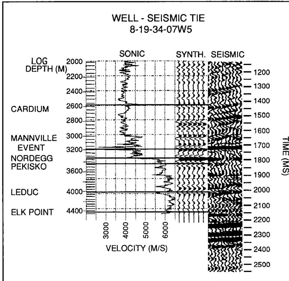
FIG. 3. Correlation of seismic data with synthetic seismogram for 8-19-34-07W5.
