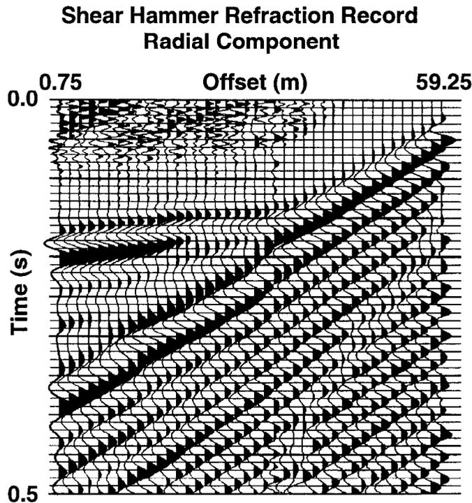
Fig. 3. Radial component refraction record. Shear hammer ( $S_H$ ) source. This is a differenced record with P-wave energy reduced and S-waves enhanced.
