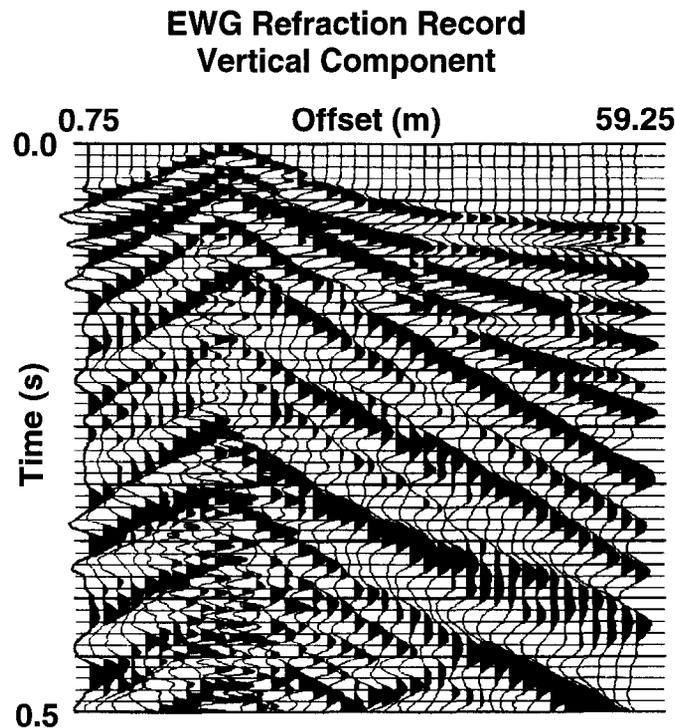
Fig. 2. Vertical component refraction record obtained using EWG device. Rayleigh waves dominate after the first breaks. The first arrivals are readily interpreted.
