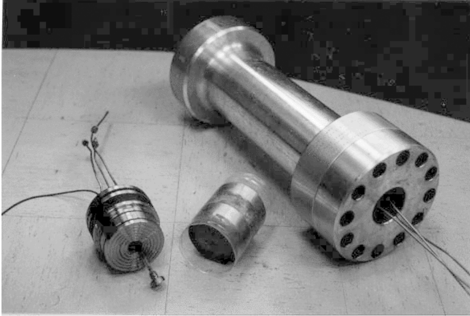
Fig. 1 The above photo shows the pressure vessel, (on the right), the sandstone core incased in plastic (center) and the stainless steel head (left). The transducer is also visible hanging out of the head.
